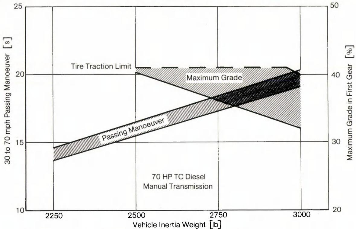
**Figure 10 Time Range for a 30 to 70 mph Passing Manoeuver and Maximum Grade as a Function of Driveline Ratio and Inertia Weight.**
