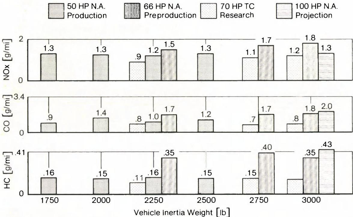
**Figure 4 Regulated Exhaust Emissions from Various Diesel Engines.**
