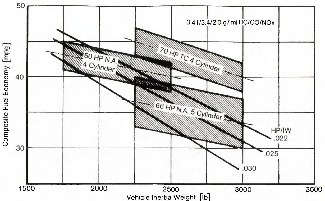
**Figure 3 Comparison of Fuel Economy of 3 Different Diesel Engines.**
