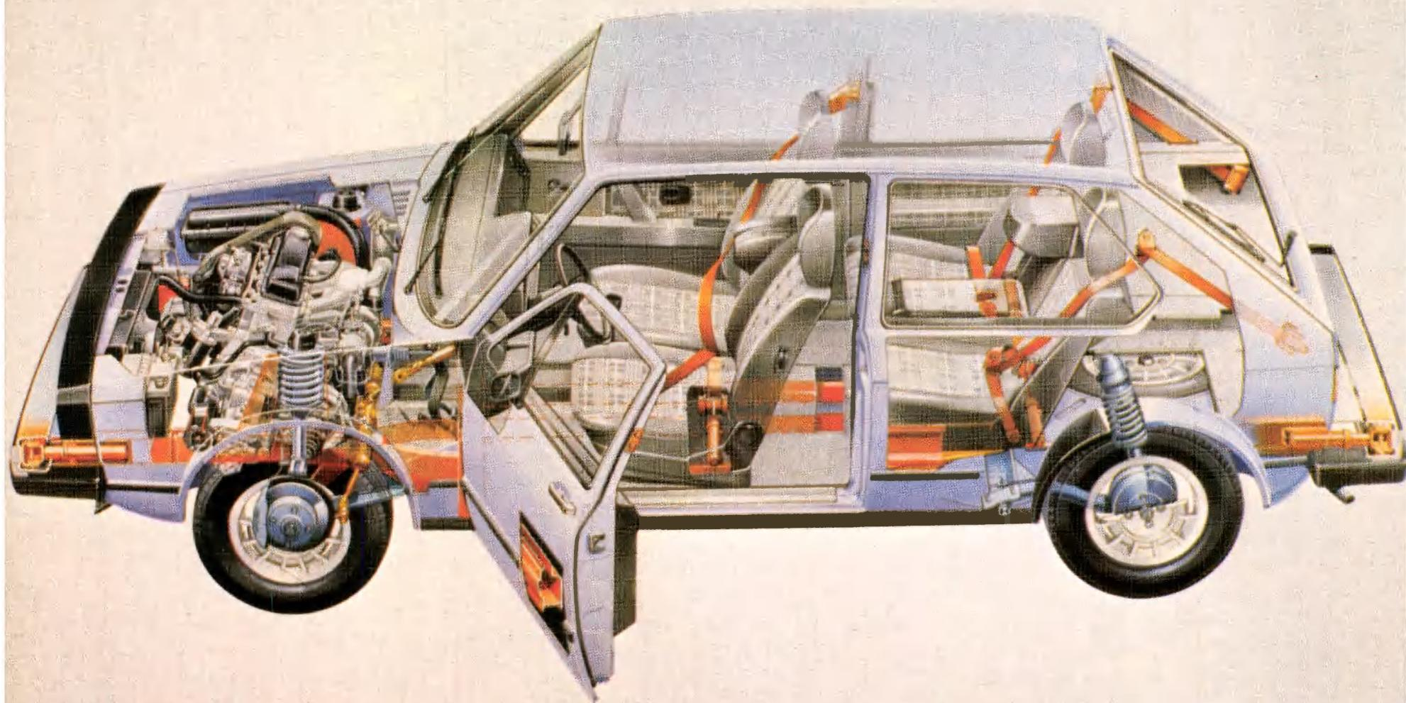
Fig. 15 Cutaway View of the VW Integrated Research Vehicle (IRVW)
