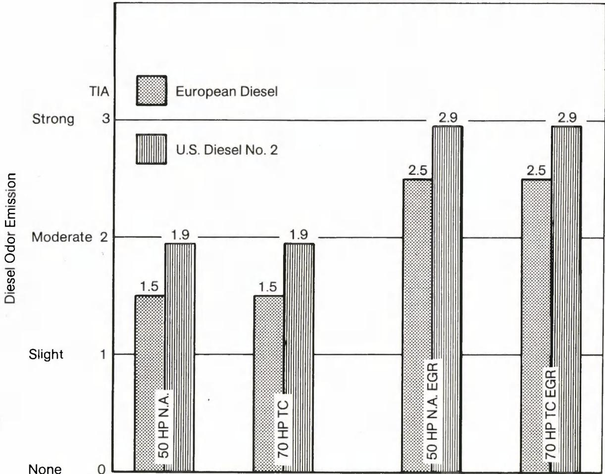
**Figure 7 Diesel Odor Emission Averaged over a City Driving Cycle Influenced by Fuel Composition and Exhaust Gas Recirculation (EGR).**
