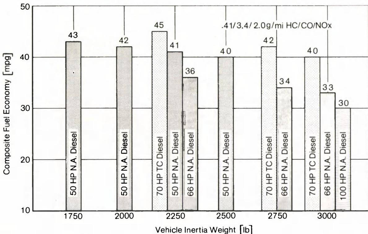
**Figure 2 Composite Fuel Economy of Various Diesel Engines Averaged over the City and Highway Driving Cycles.**
