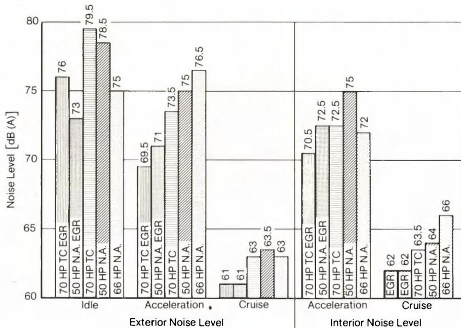
**Figure 8 Noise Emission by Various Engine/Vehicle Systems Measured at a Speed of 30 mph and at a Distance of 15 m (50 ft) according to SAE J 986 a.**
