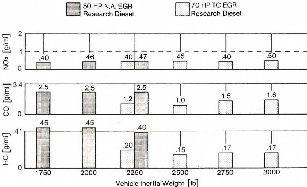
**Figure 5 Regulated Exhaust Emissions of Two Diesel Engines with Controlled Exhaust Gas Recirculation (Preliminary Data).**
