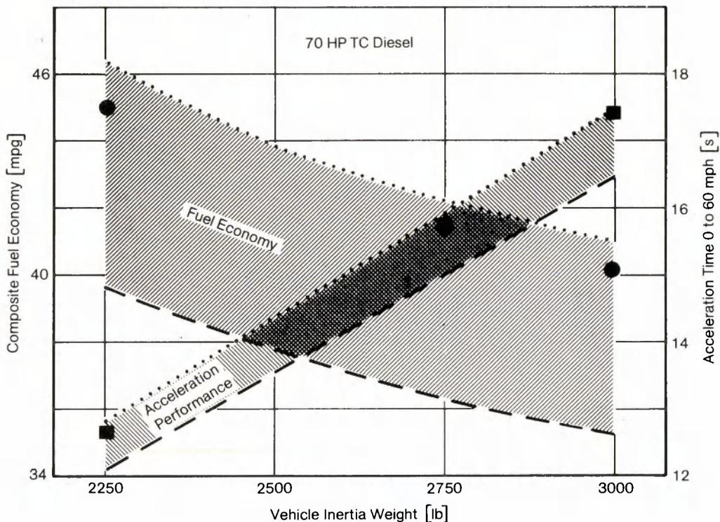
**Figure 9 Fuel Economy and Acceleration Performance as a Function of Drivetrain Ratio and Weight.**
