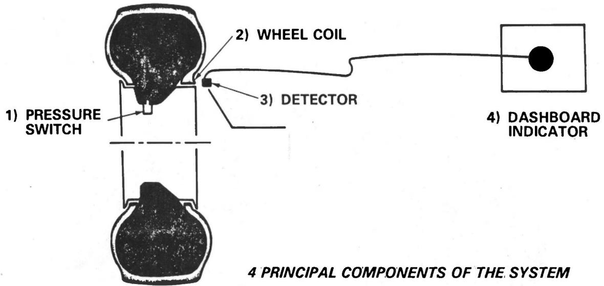
Figure 94 GOODYEAR LOW TIRE PRESSURE WARNING SYSTEM
