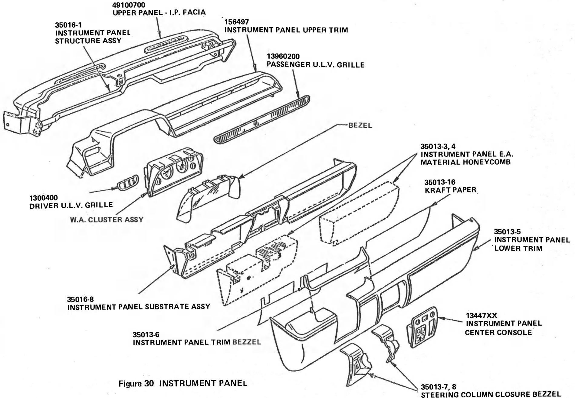
Figure 30 INSTRUMENT PANEL
