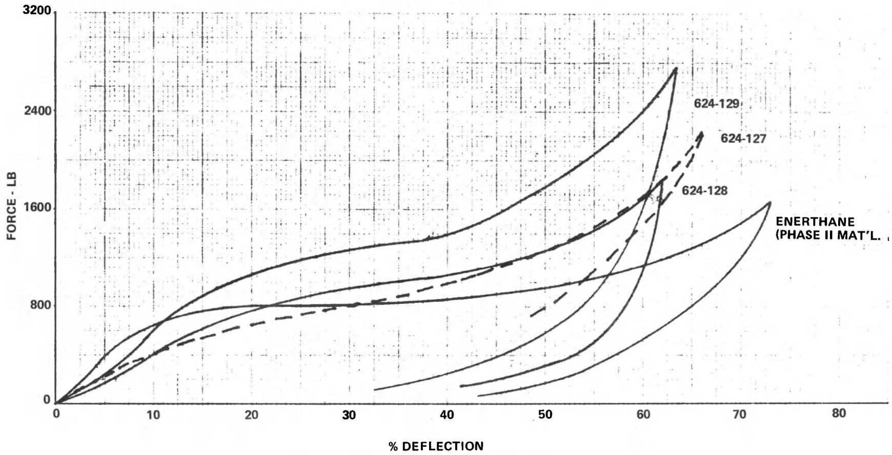
Figure 22 PERFORMANCE OF BUMPER ENERGY ABSORBING FOAM
