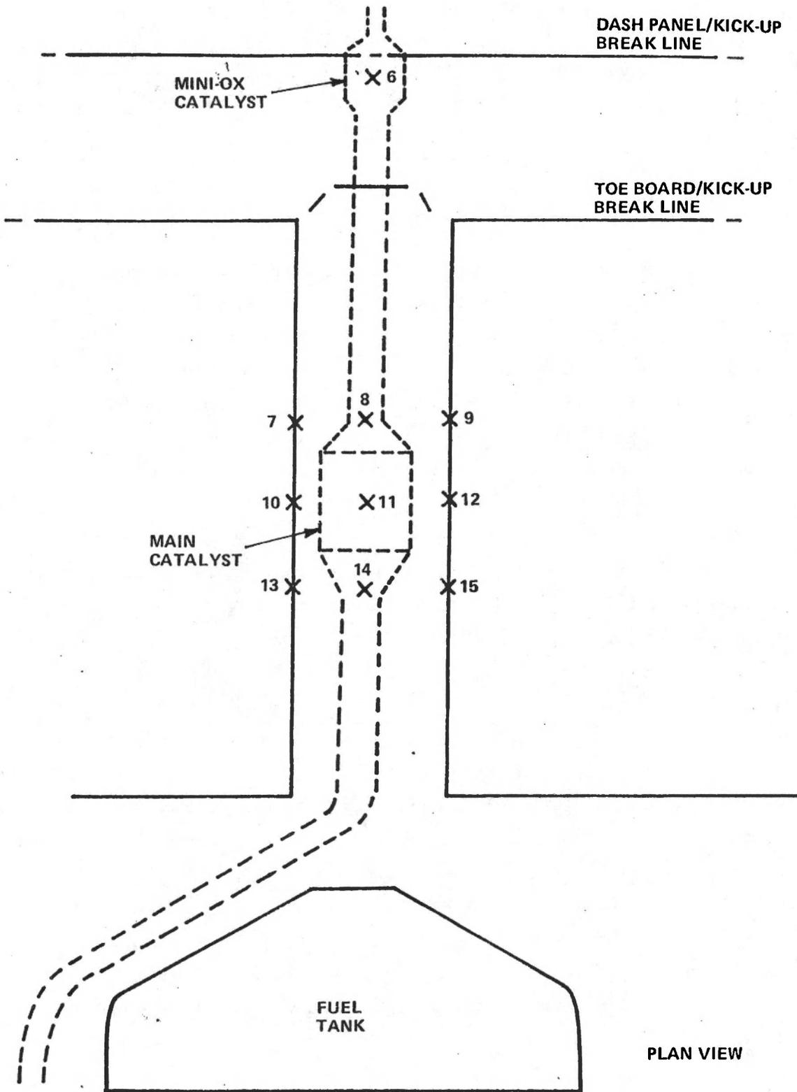
Figure 84 FLOOR PAN THERMOCOUPLE LOCATIONS
