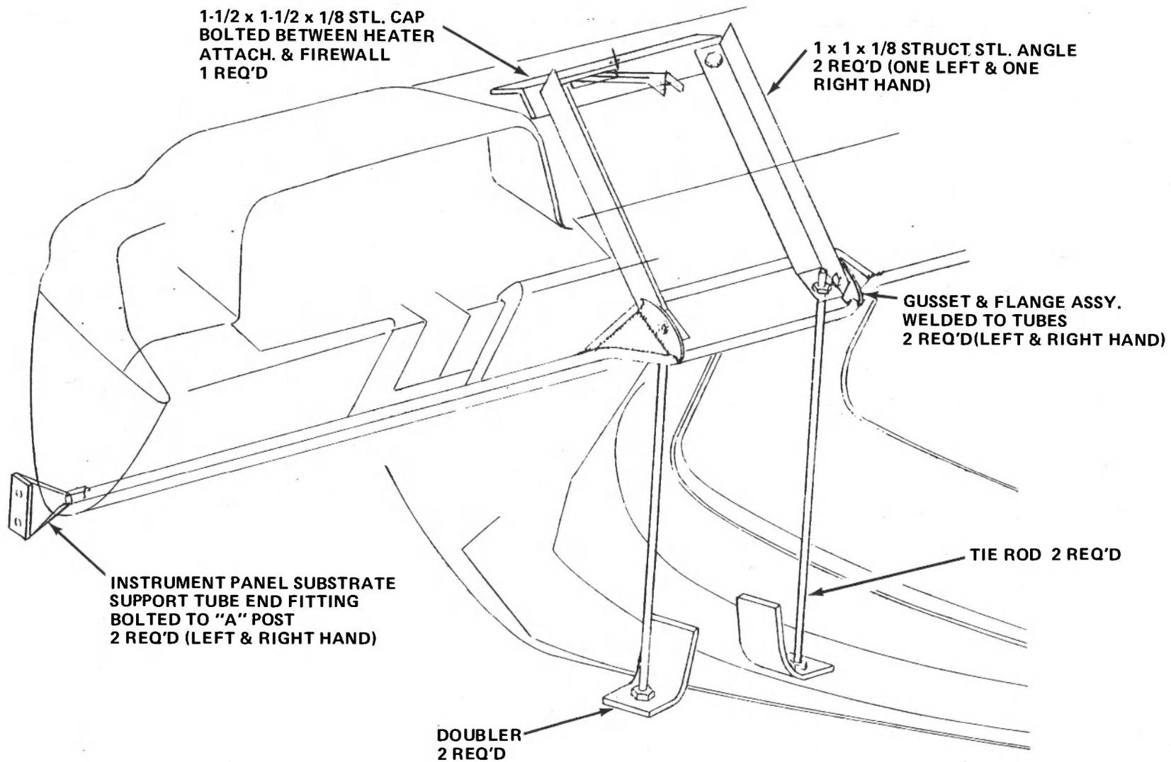
Figure 31 RSV INSTRUMENT PANEL SUPPORT STRUCTURE MODIFICATIONS
