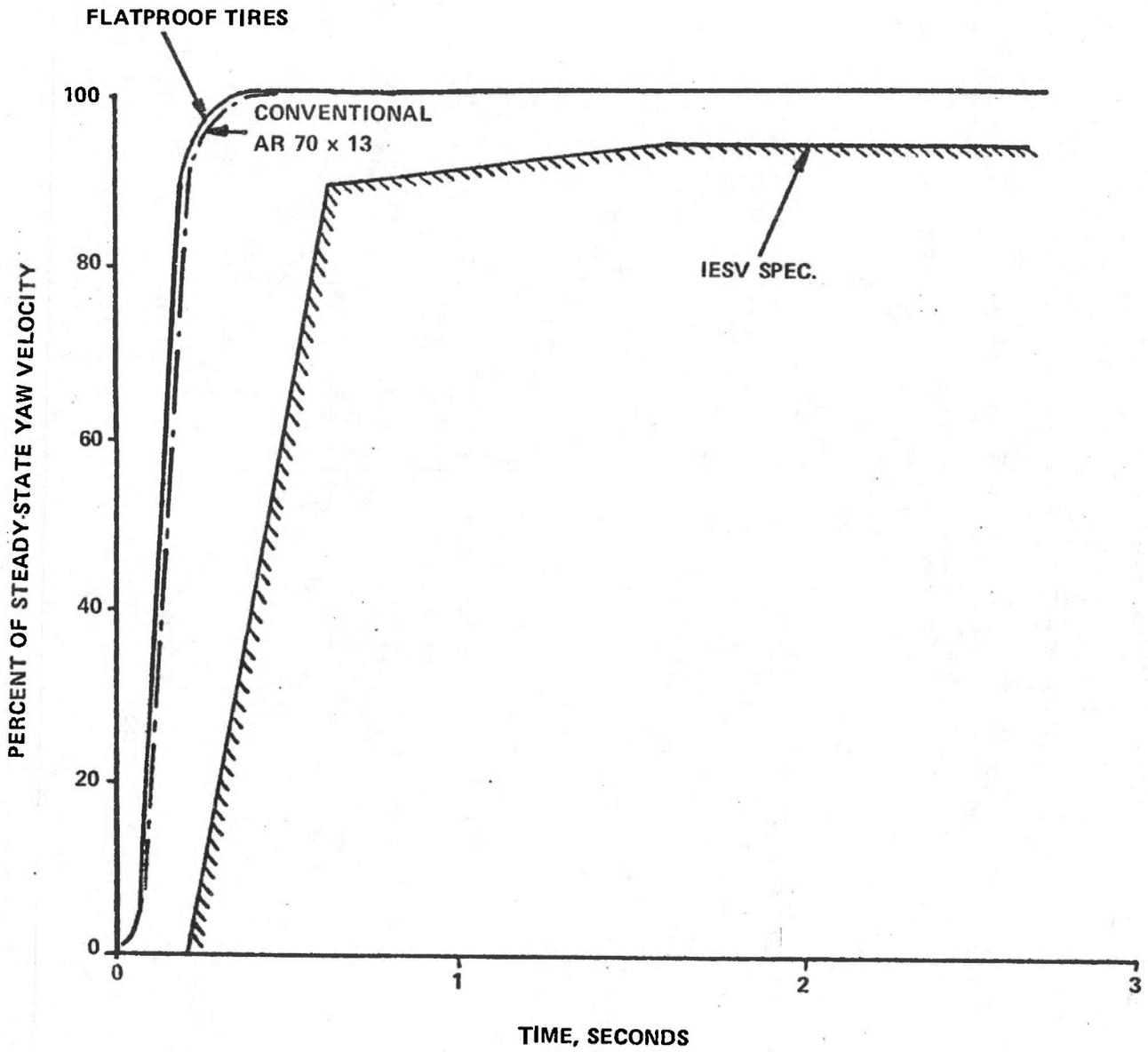
Figure 77 CALCULATED TRANSIENT RESPONSE, 25 MPH, 0.4 G CONVENTIONAL VS. FLATPROOF TIRES
