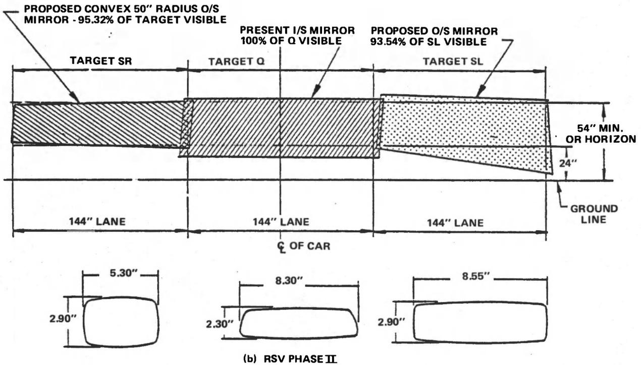
Figure 51 INDIRECT VISIBILITY – MIRROR TARGET PLANE
