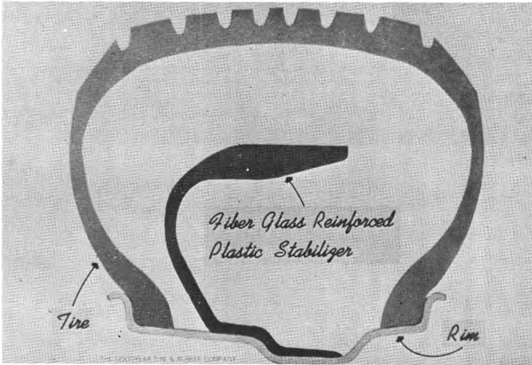
Figure 89 14 INCH FLATPROOF TIRE WITH INTERNAL STABILIZER
