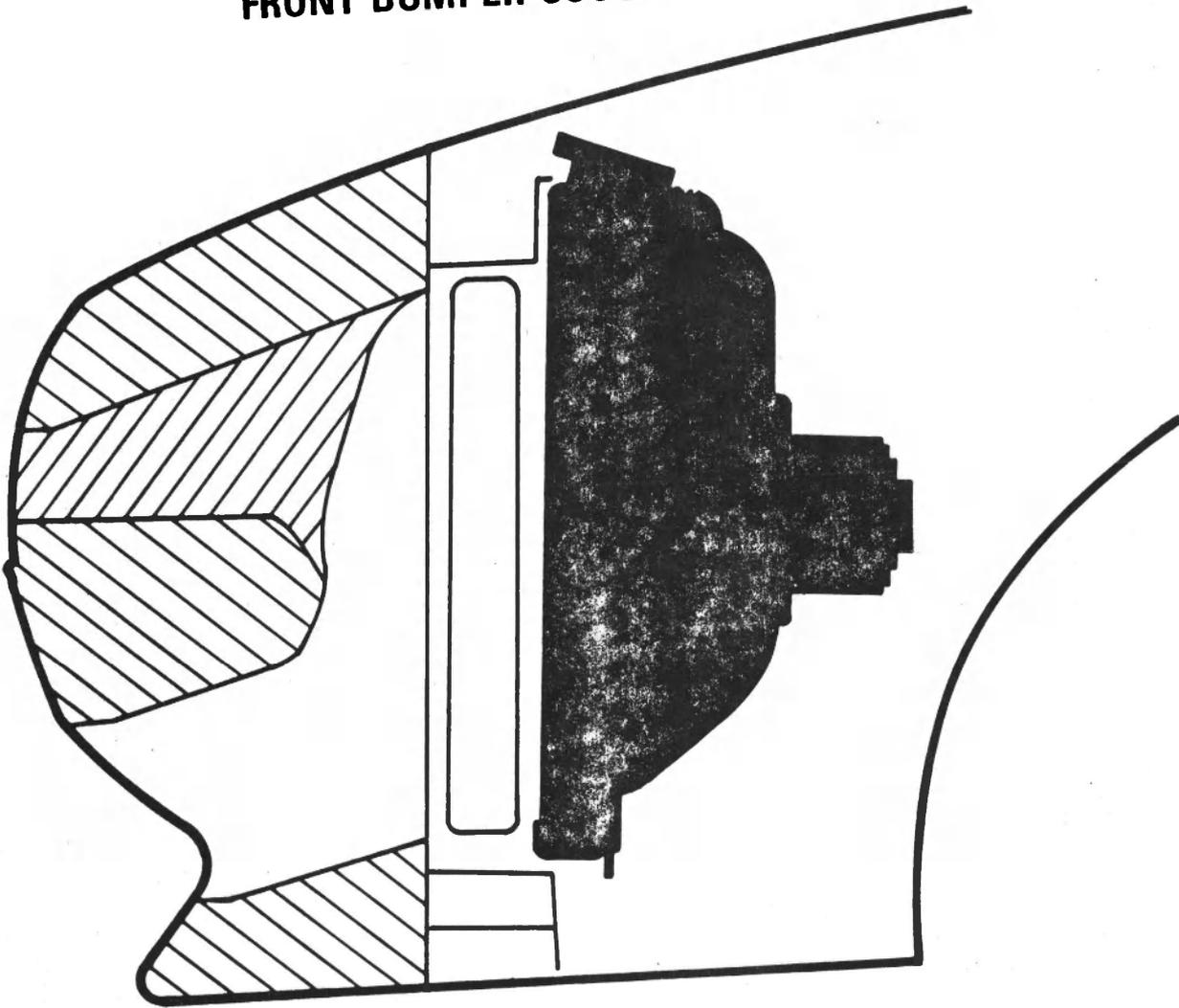
**Figure 66 RADIATOR DUCTING**
