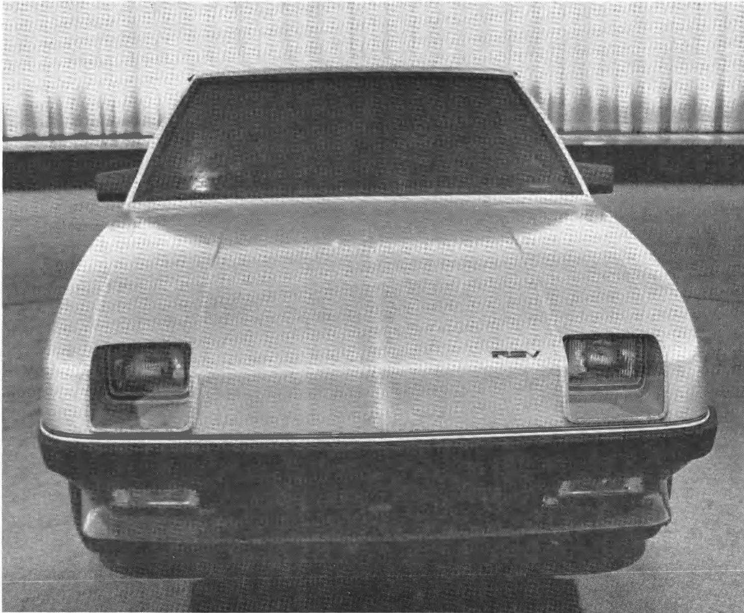
Figure 108 RSV FRONT WITHOUT COOLING SLOTS
