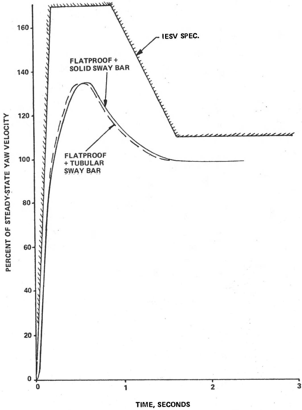
Figure 80 SOLID VS. TUBULAR SWAY BAR CALCULATED TRANSIENT RESPONSE
