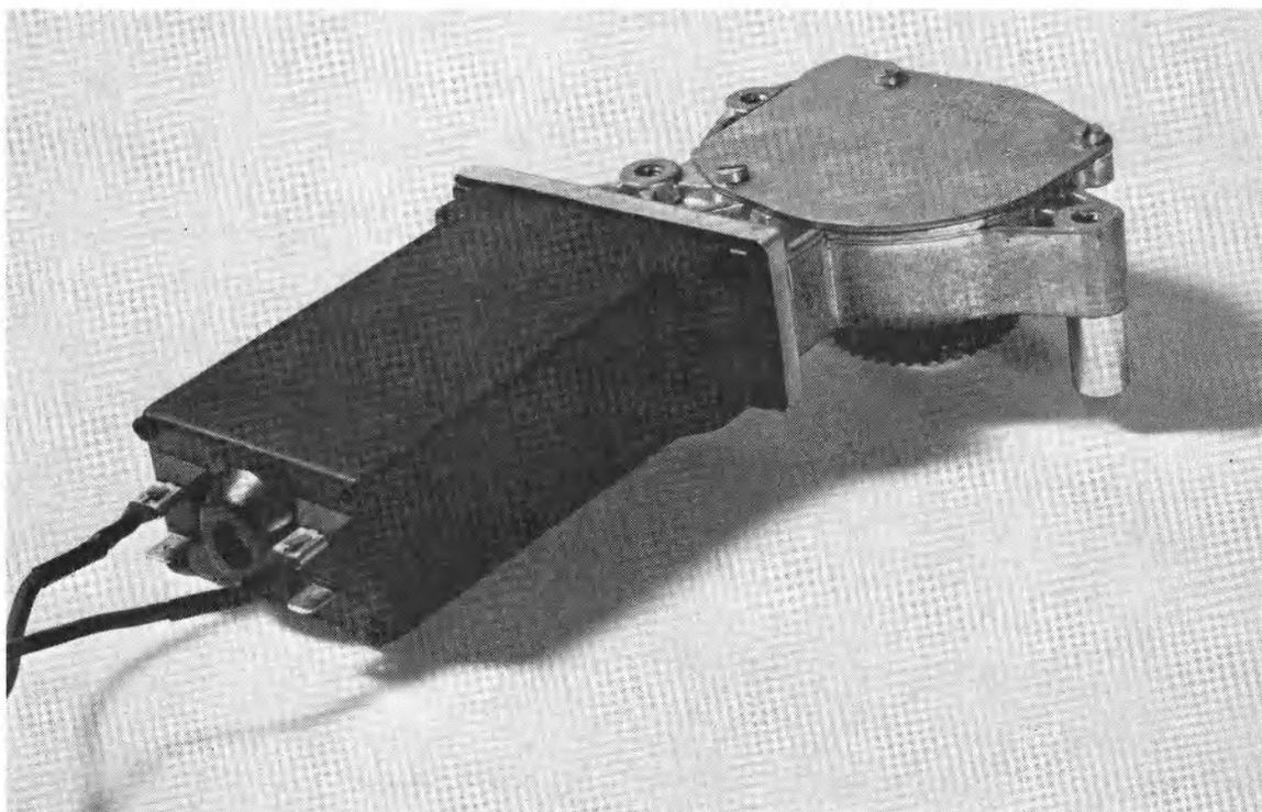
**Figure 44** AUTOMATIC BELT DEPLOYMENT MOTOR
