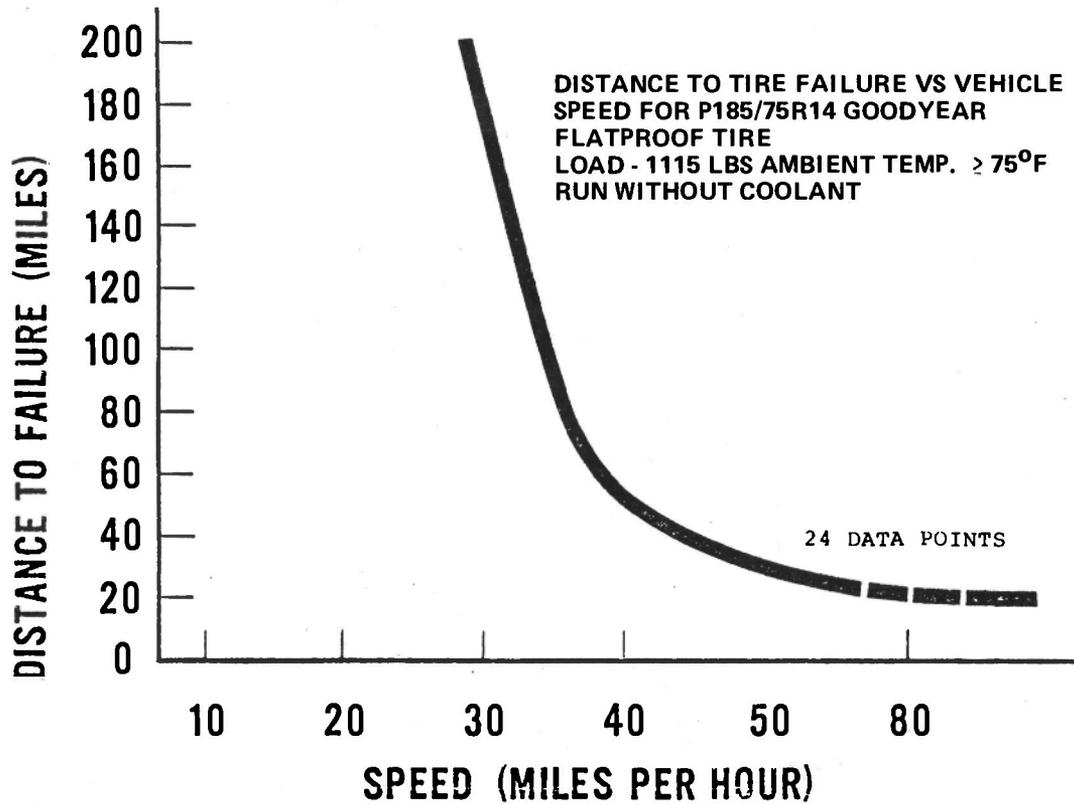
Figure 92 GOODYEAR FLATPROOF DATA WITHOUT COOLANT
