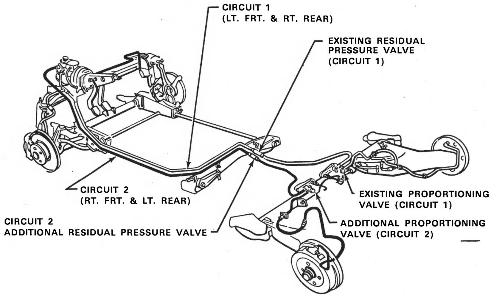
Figure 82 BRAKE LINE ROUTING FOR PHASE III RSV WITH DIAGONAL SPLIT SYSTEM
