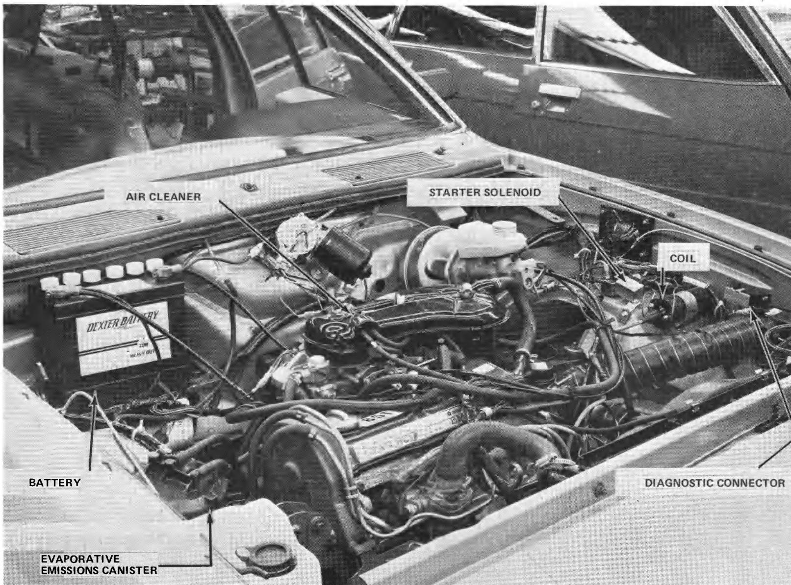
Figure 61 RSV ENGINE COMPARTMENT
