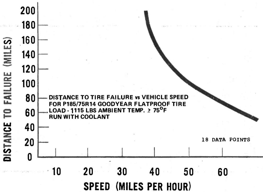
Figure 91 GOODYEAR FLATPROOF DATA WITH COOLANT
