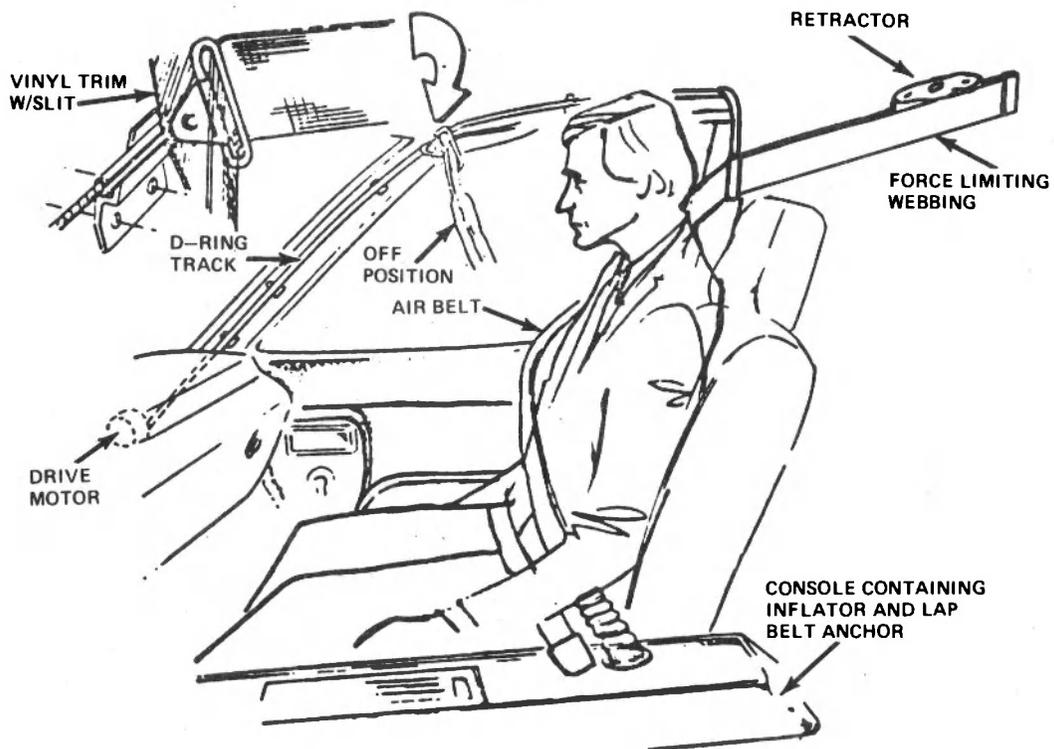
**Figure 40 INFLATABLE SHOULDER BELT – PHASE III**
