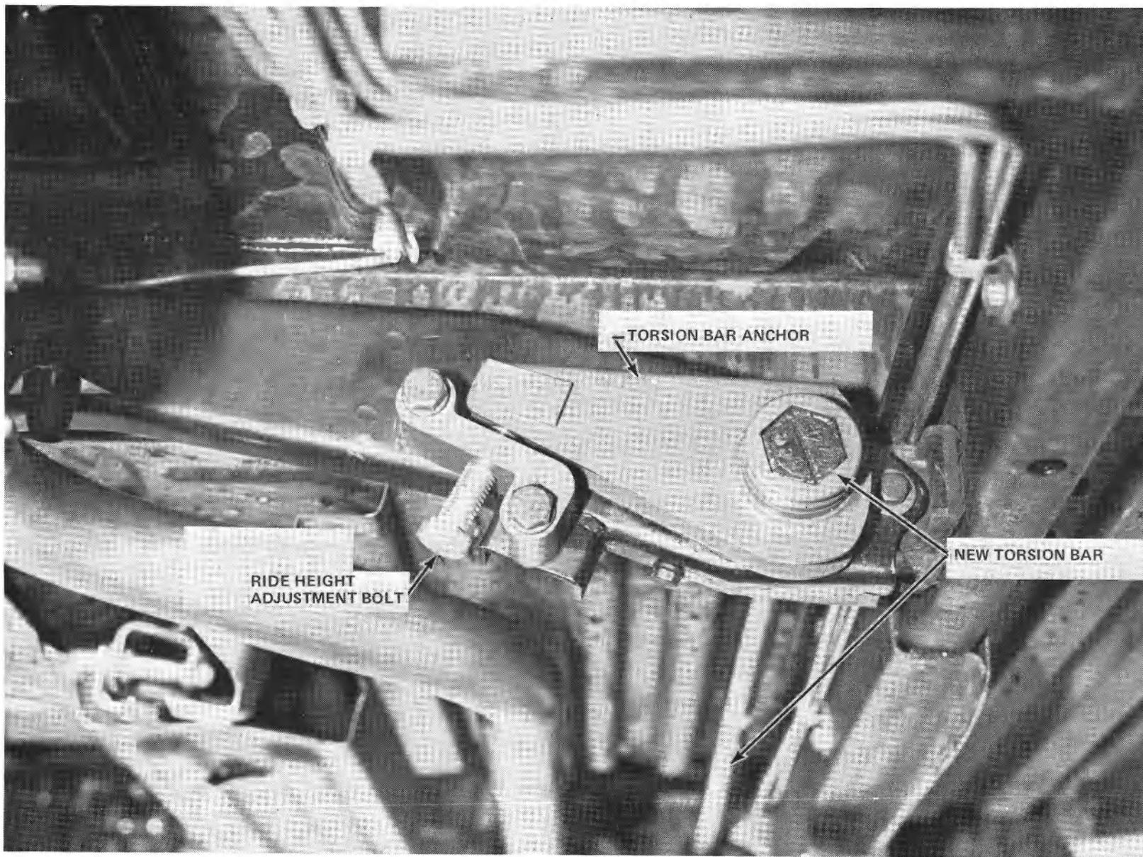
Figure 75 RSV REAR TORSION BAR ANCHOR
