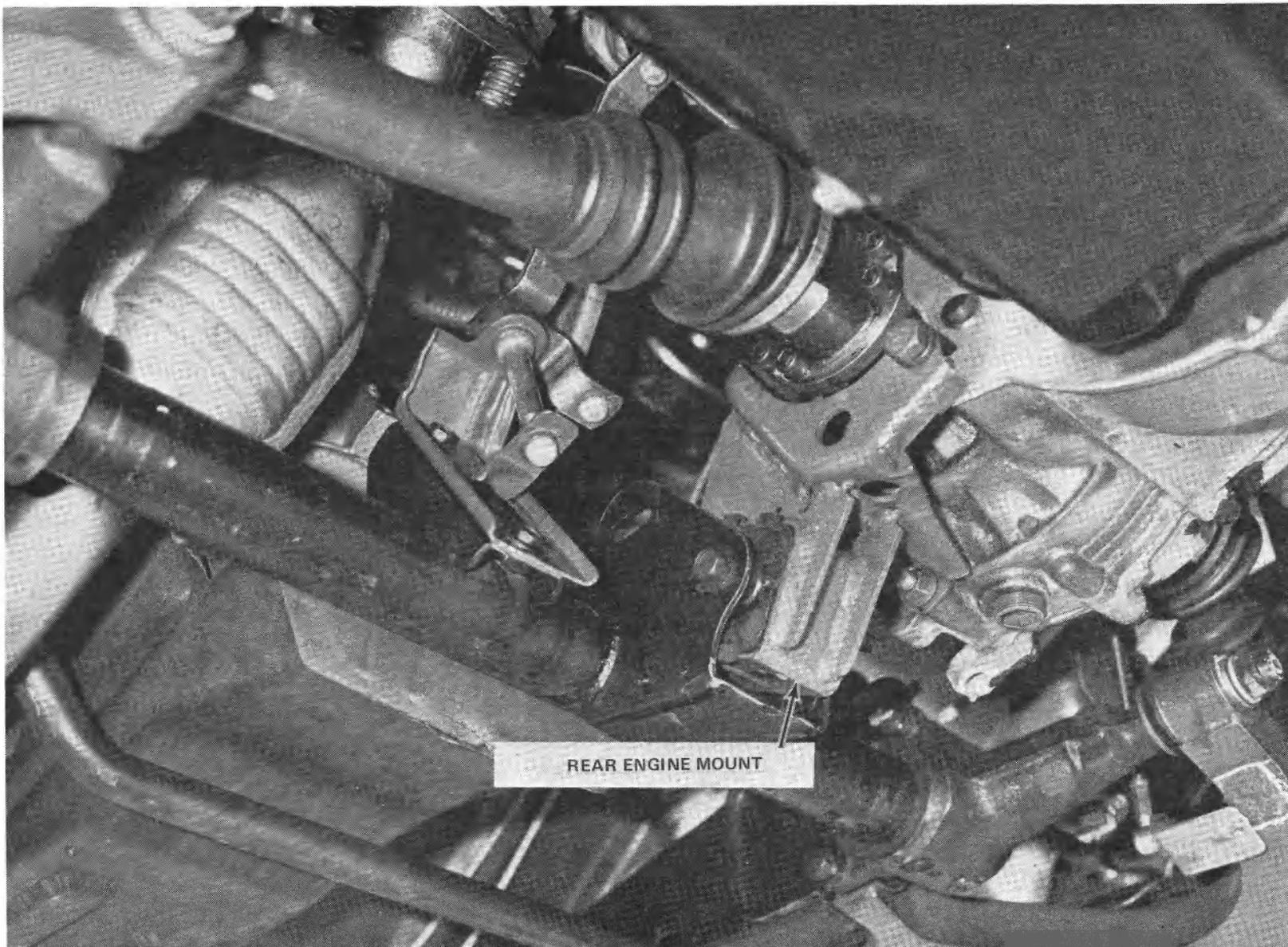
Figure 60 REAR ENGINE MOUNT
