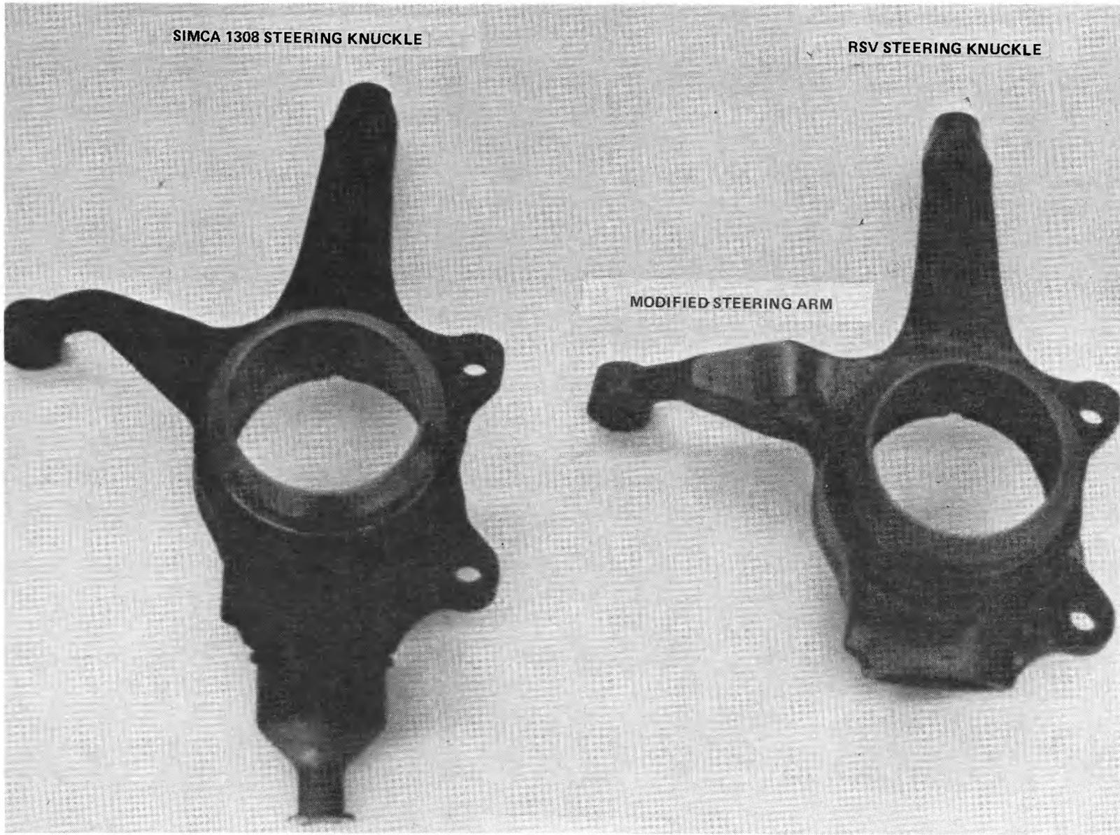
Figure 68 STEERING KNUCKLE MODIFICATION
