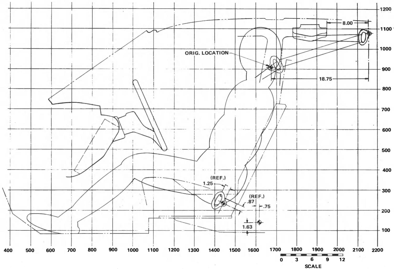
Figure 39 RSV AIR BELT ANCHOR POINT GEOMETRY
