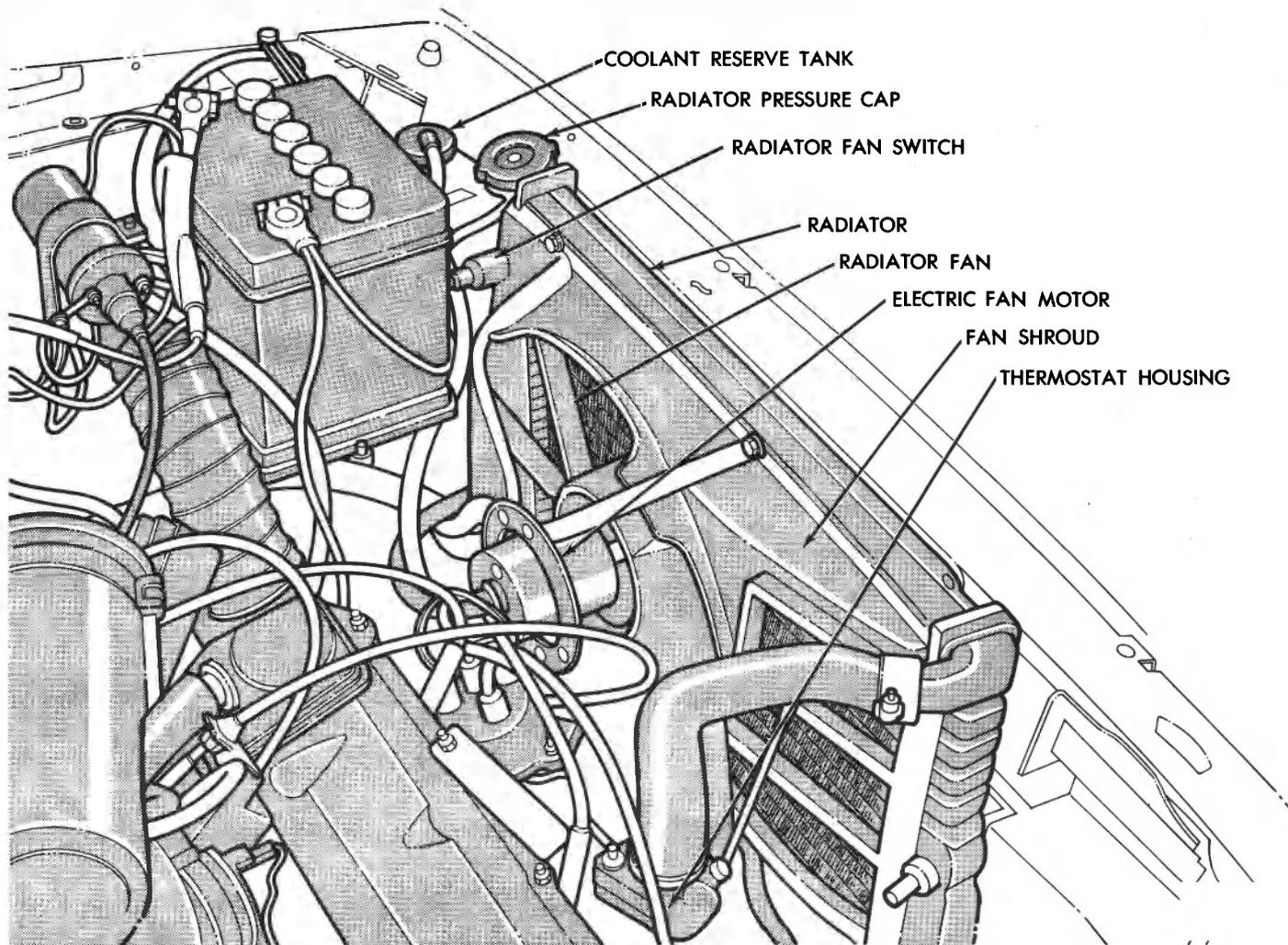
Figure 65 COOLING SYSTEM
