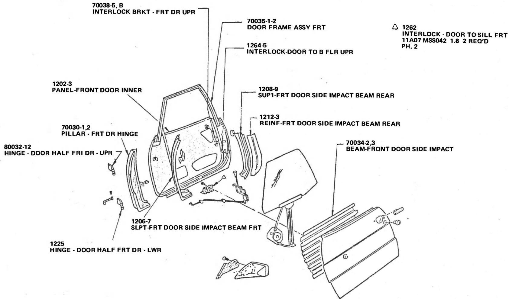
Figure 18 FRONT DOOR STRUCTURE
