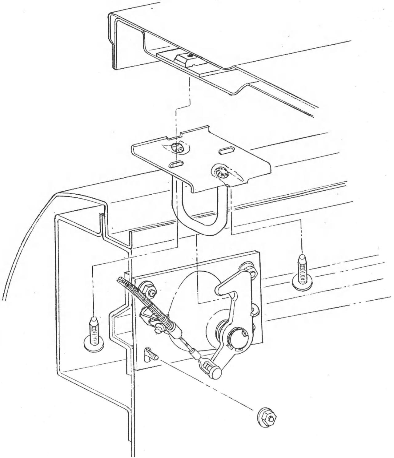
Figure 23 SECONDARY HOOD LATCH – PHASE III
