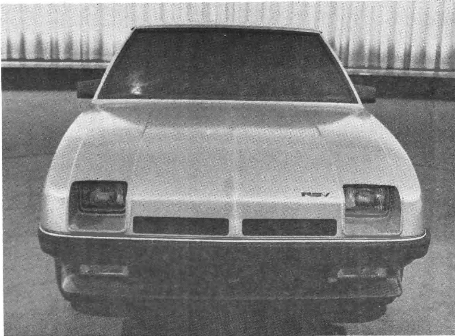
Figure 107 RSV FRONT WITH UPPER COOLING SLOTS
