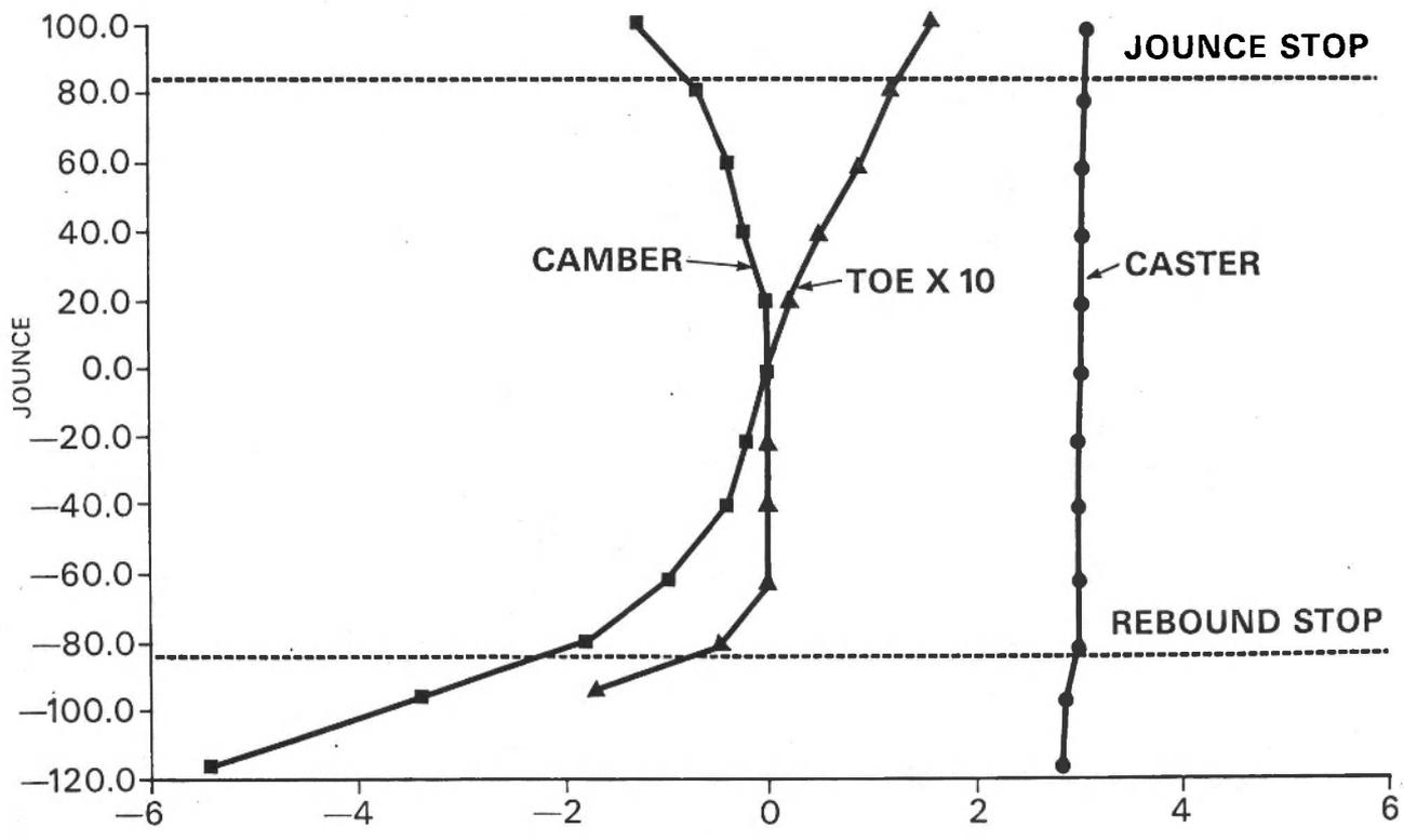
Figure 71 RSV FRONT SUSPENSION GEOMETRY
