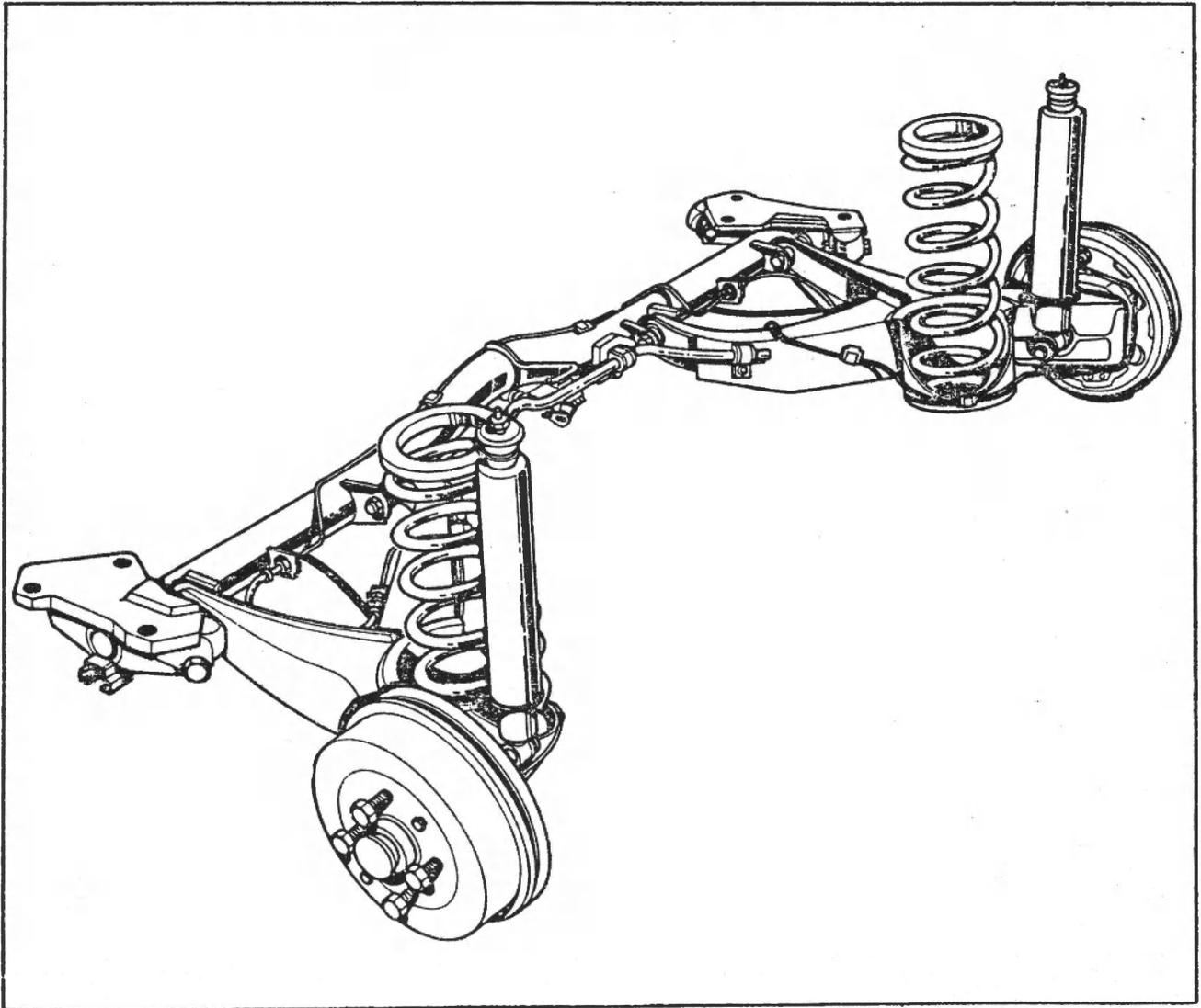
**Figure 76 SIMCA INDEPENDENT TRAILING ARM REAR SUSPENSION**
