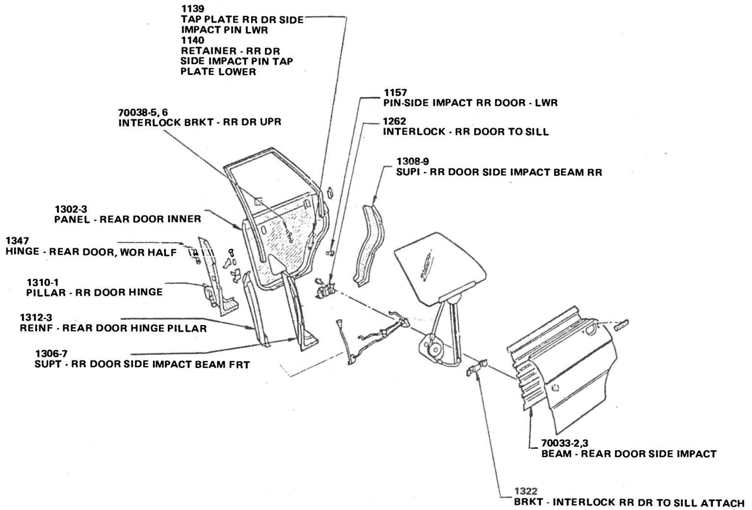
Figure 19 REAR DOOR STRUCTURE
