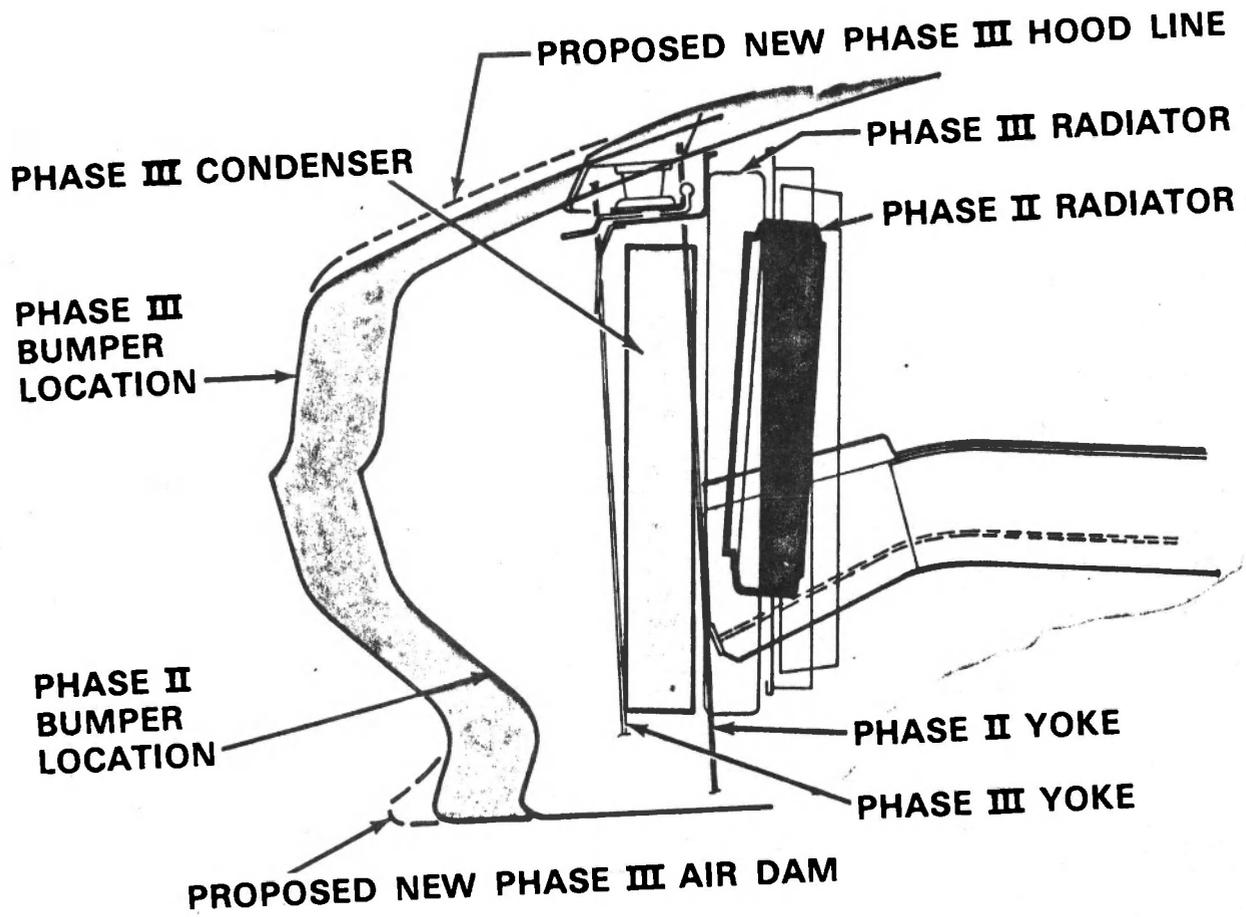
Figure 64 CHANGES IN RADIATOR POSITION, PHASE II TO PHASE III
