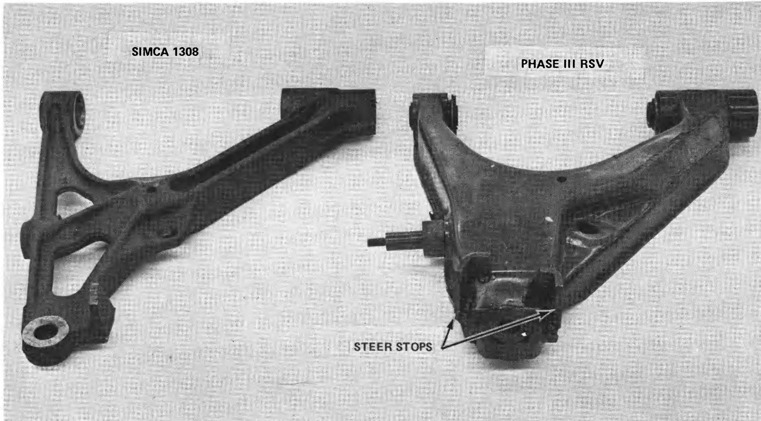
Figure 72 FRONT SUSPENSION LOWER CONTROL ARM
