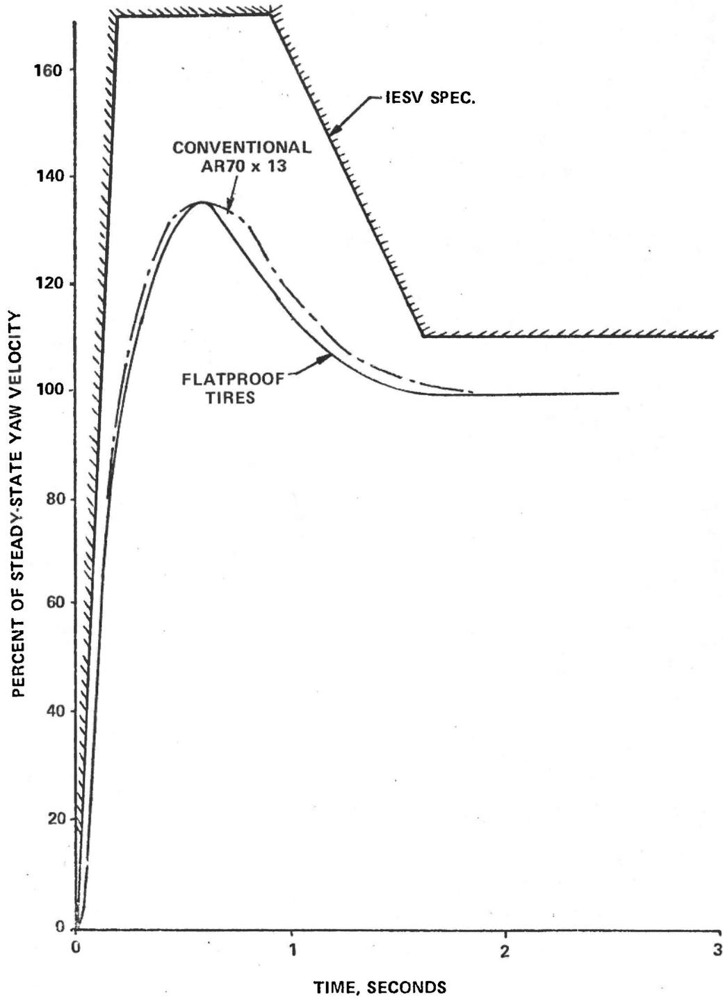
Figure 78 CONVENTIONAL VS. FLATPROOF TIRES CALCULATED TRANSIENT RESPONSE, 70 MPH, 0.4 G
