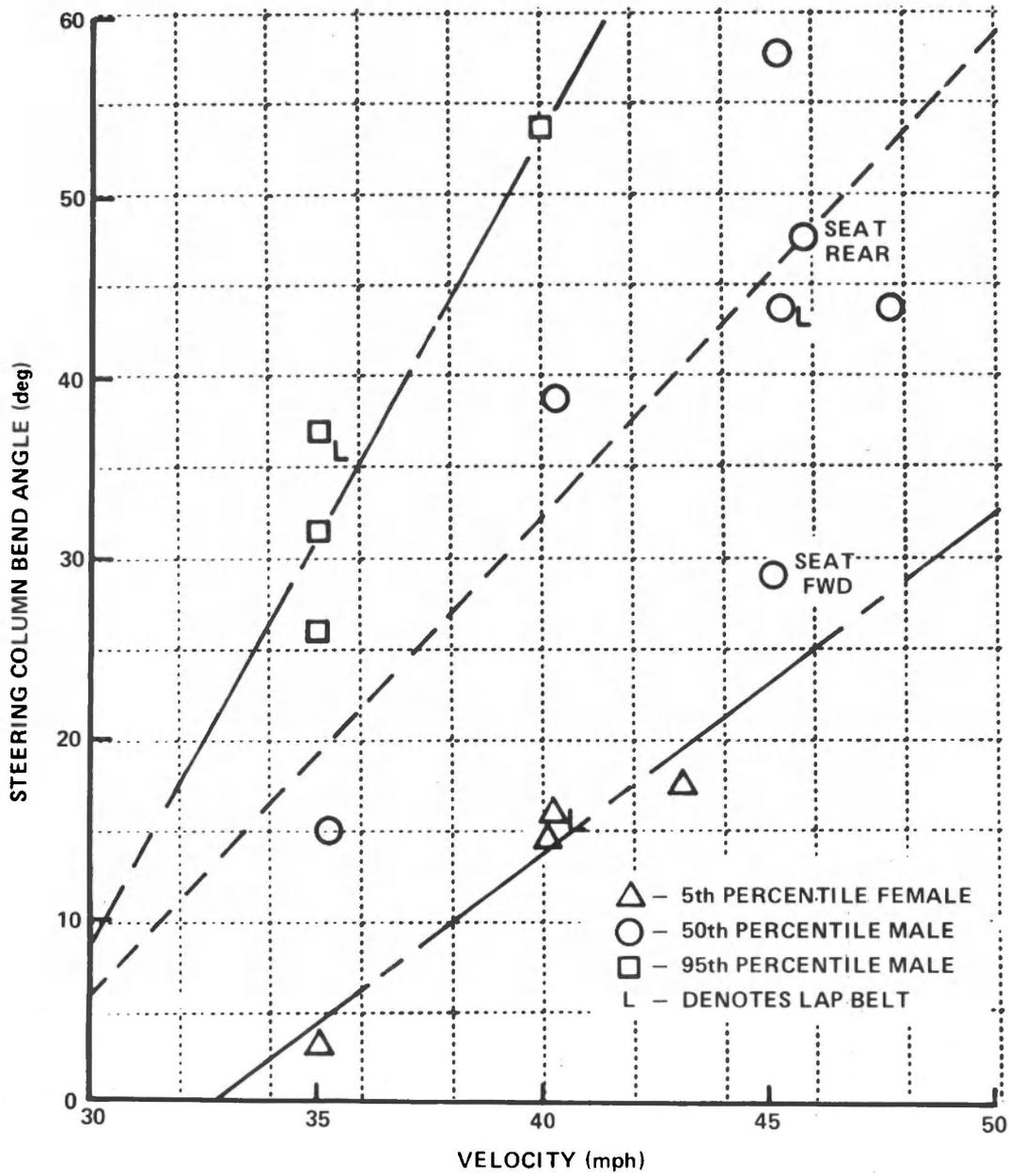
Figure 46 COLUMN BEND DEPENDENCE ON SPEED OF SLED IMPACT
