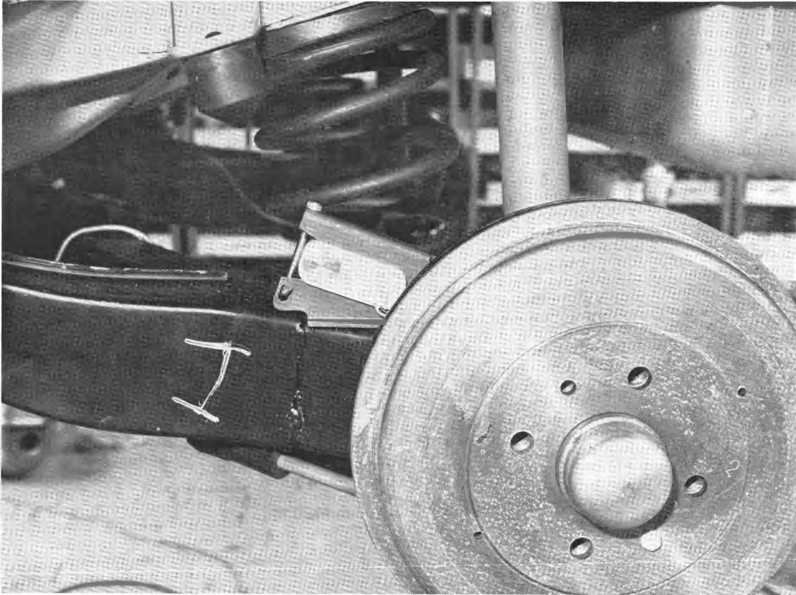
Figure 97 DETECTOR INSTALLED ON LEFT REAR TRAILING ARM
