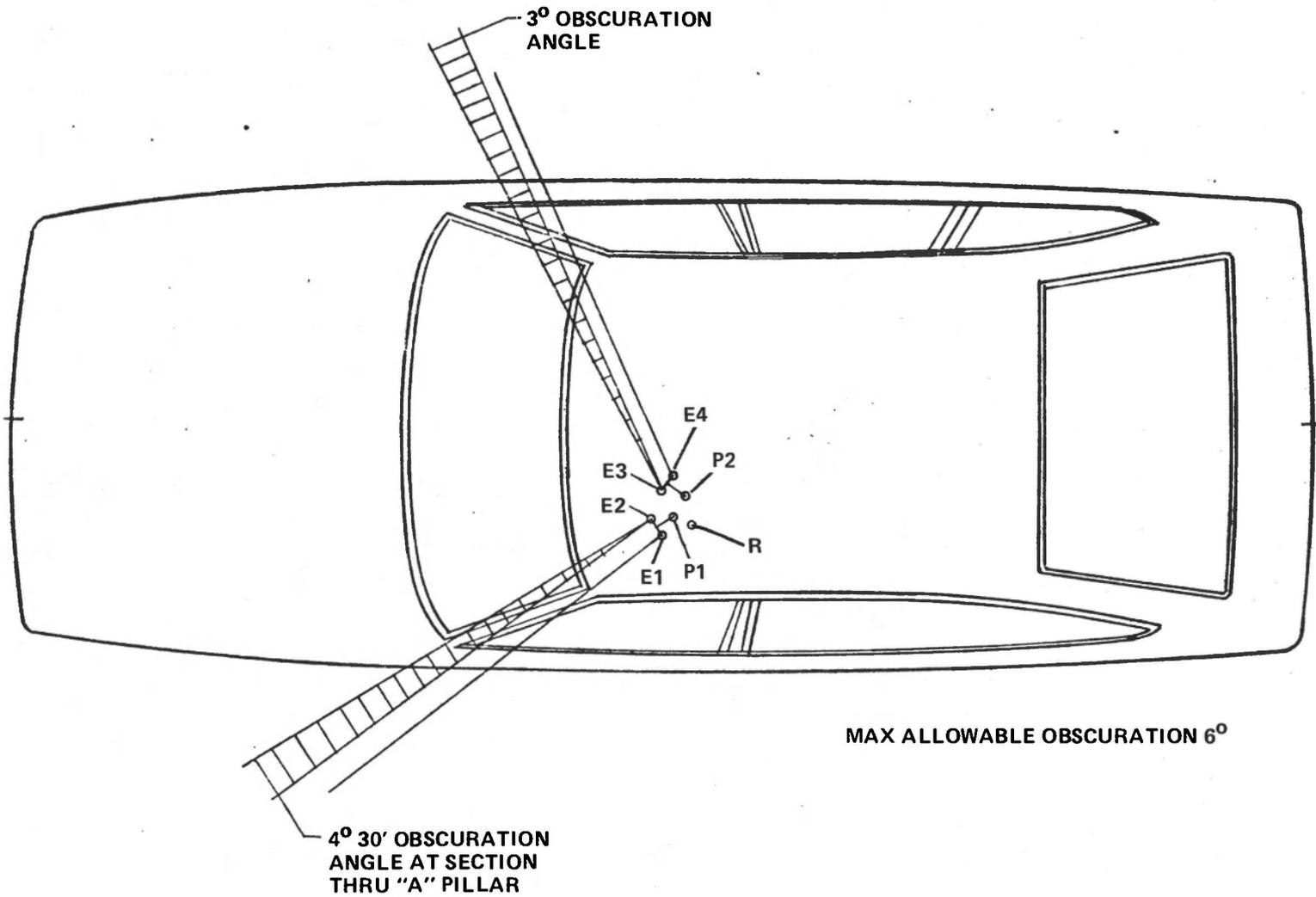
Figure 49 BINOCULAR VISIBILITY THRU "A" PILLAR
