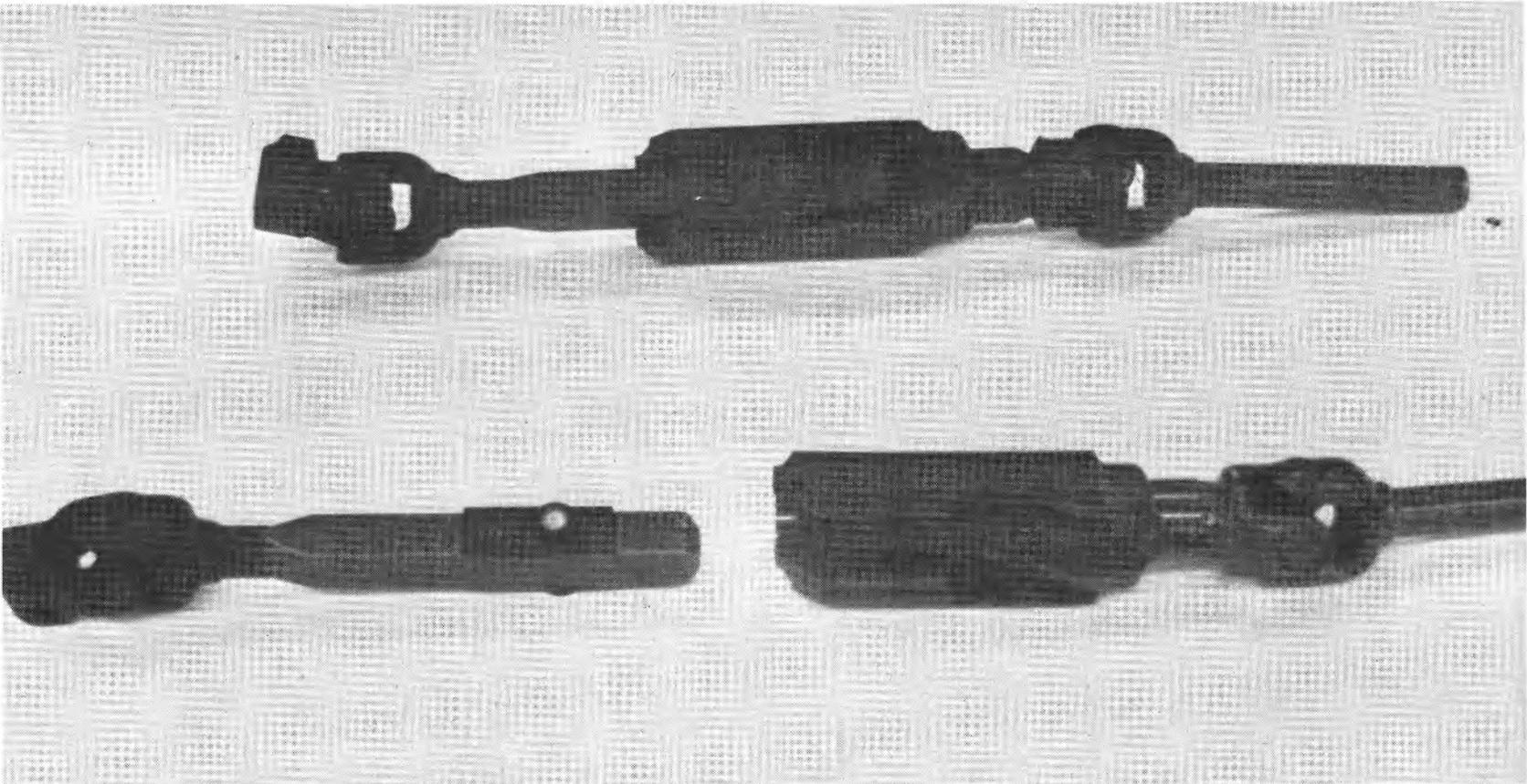
Figure 69 DE-COUPLING INTERMEDIATE STEERING SHAFT
