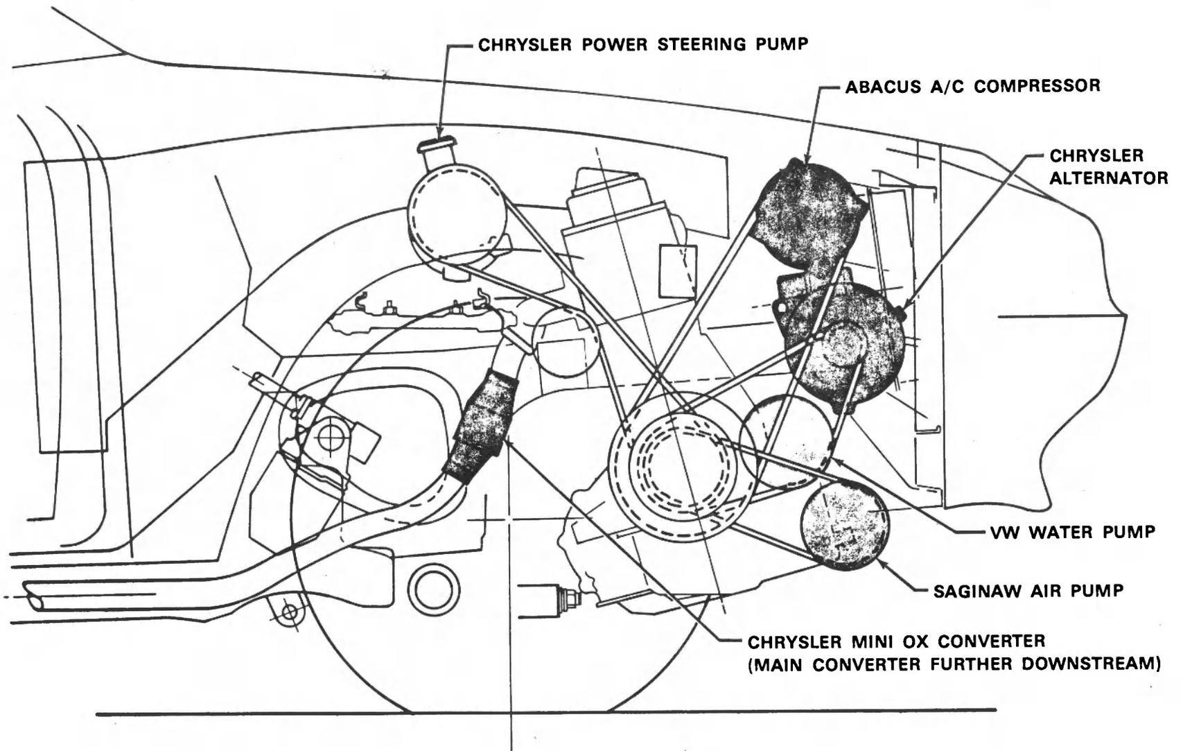
Figure 58 ENGINE COMPARTMENT & BELT DRIVE SYSTEM
