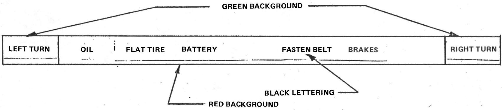
Figure 32 INSTRUMENT CLUSTER WARNING LAMPS
