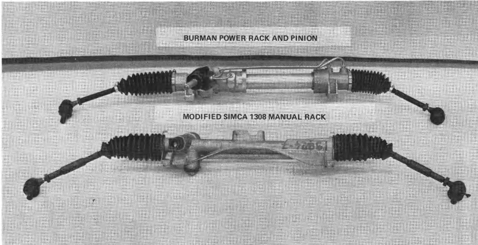
Figure 67 MODIFIED STEERING RACKS
