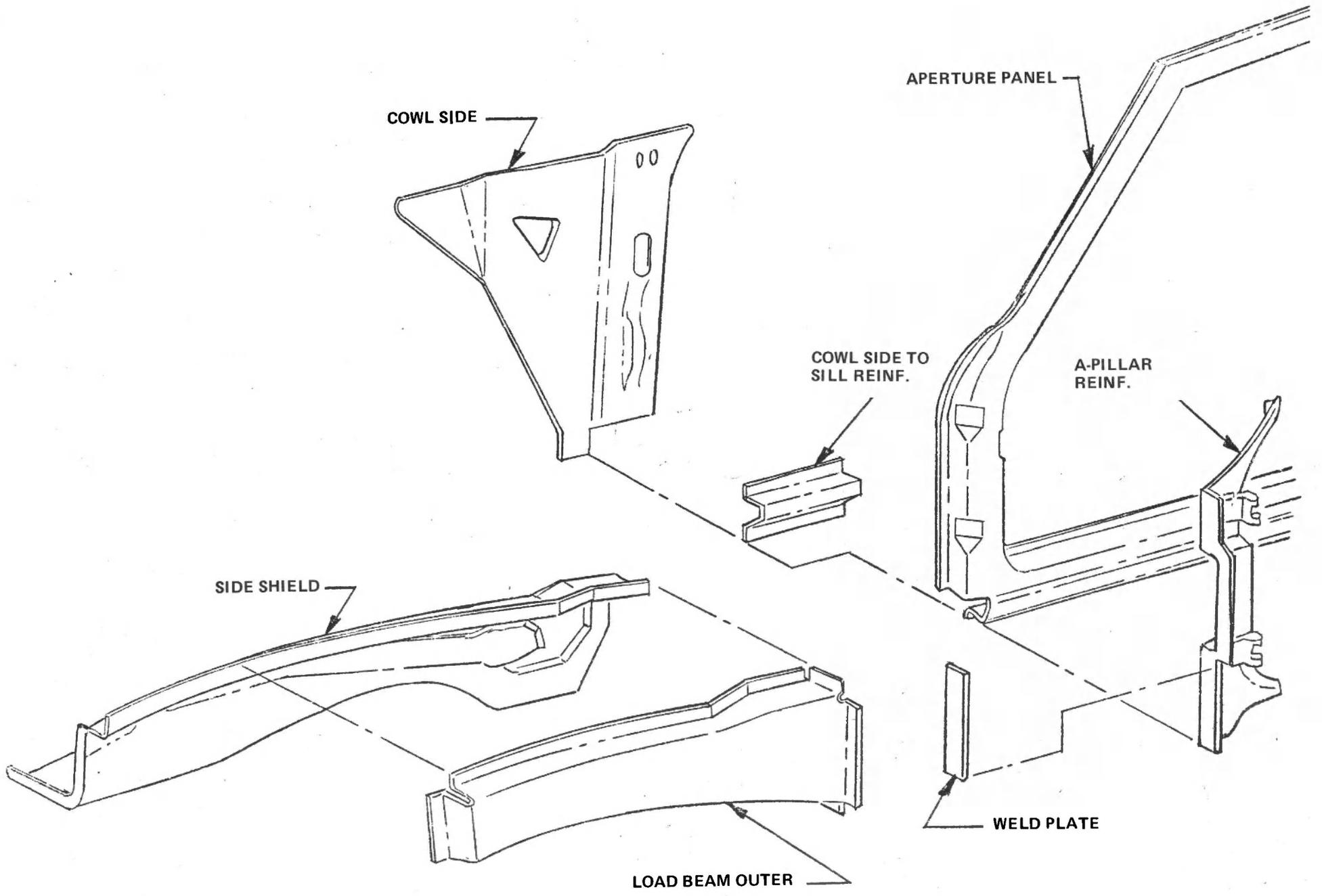
Figure 14 UPPER LOAD BEAM CONSTRUCTION – PHASE III
