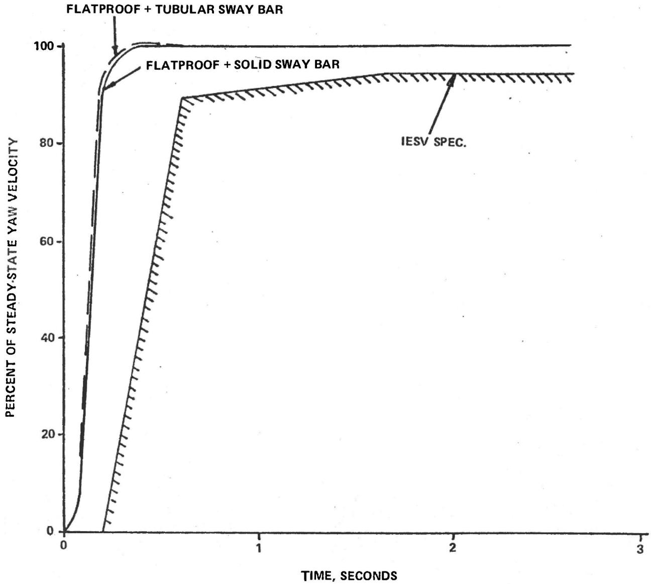
Figure 79 SOLID VS. TUBULAR SWAY BAR CALCULATED TRANSIENT RESPONSE
