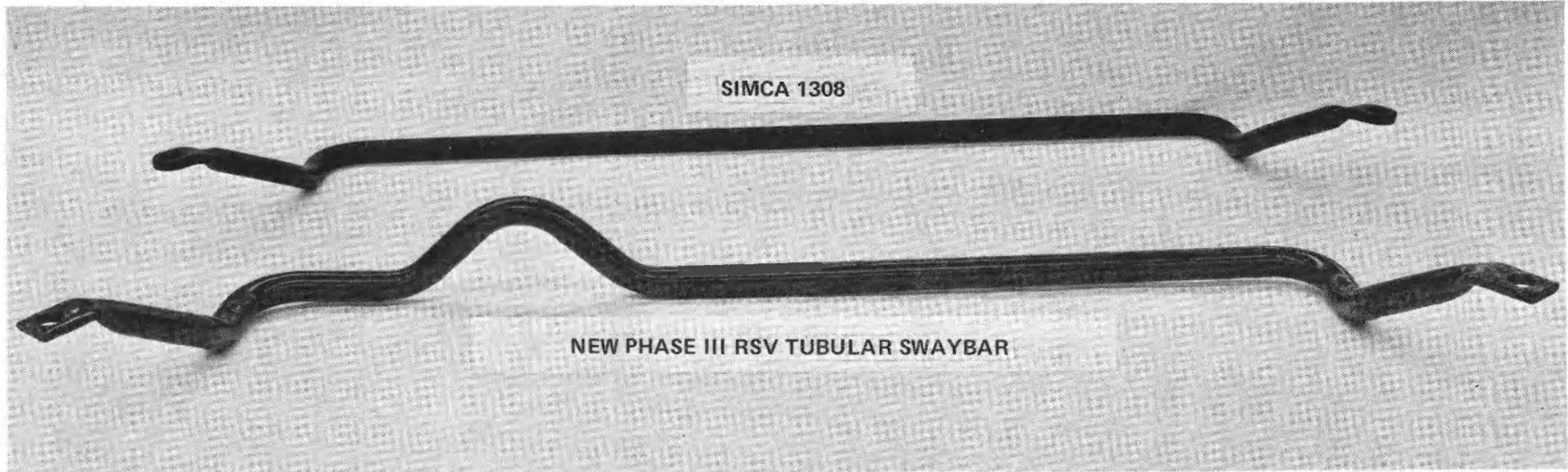
Figure 74 FRONT SWAYBAR
