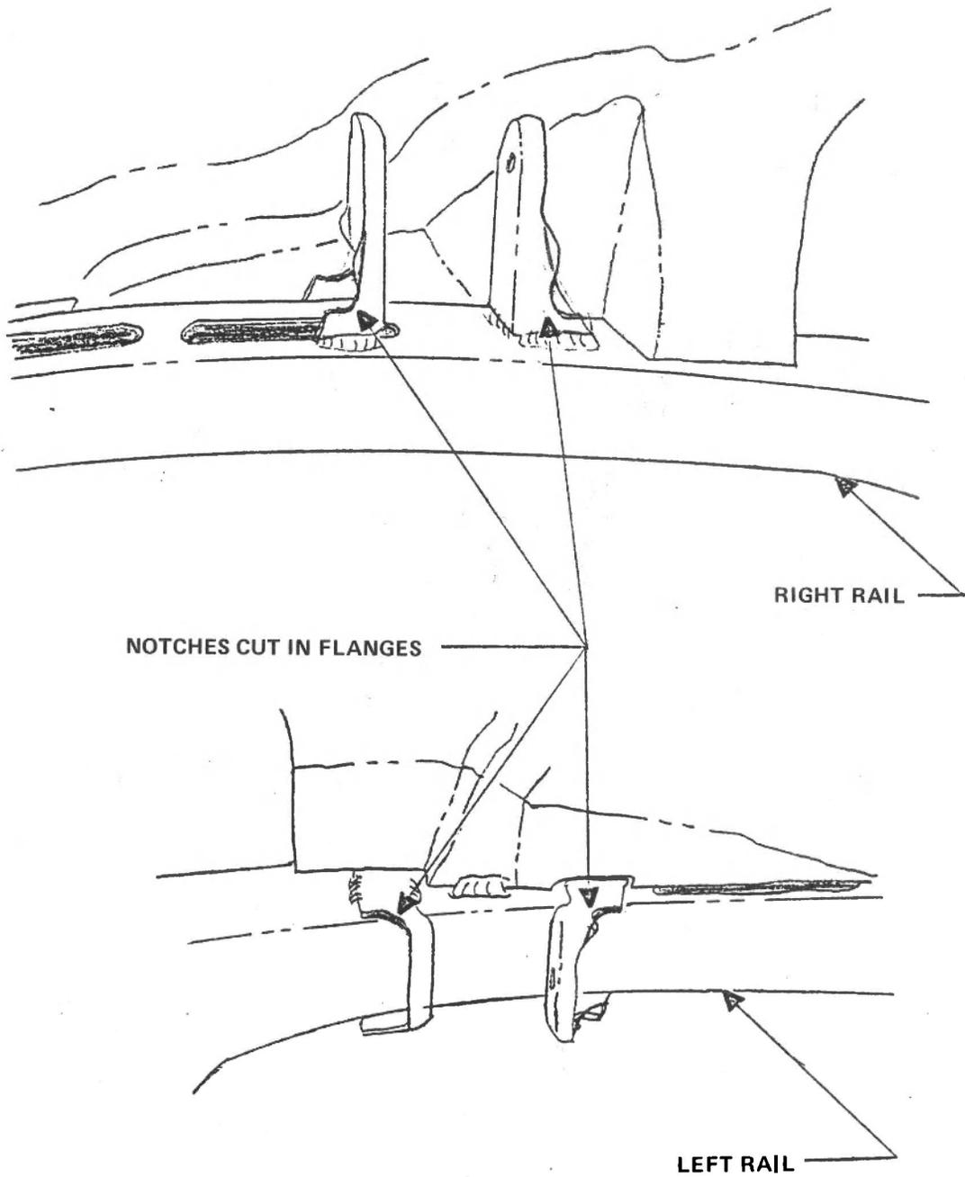
**Figure 12 ENGINE MOUNT MODIFICATIONS**
