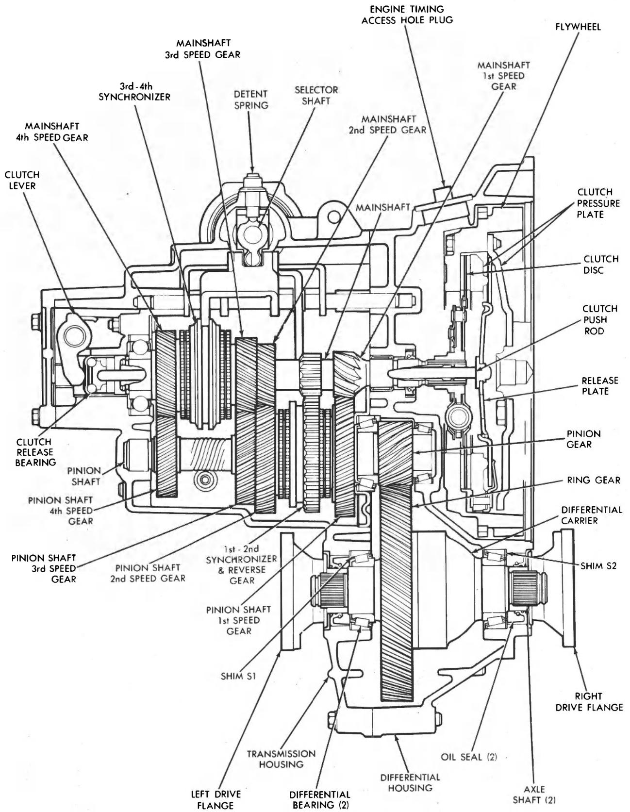
**Figure 62**      **MANUAL TRANSAXLE SCHEMATIC**
