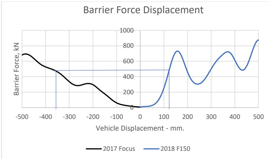
**Figure 12. Stiffness comparison of the Focus vs F 150**
