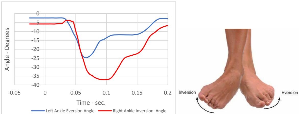
**Figure 10. Foot and Ankle Eversion/Inversion Angle Test 9500**
