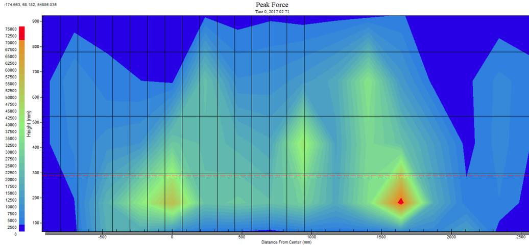
**Figure 16a. 2017 Focus 10068 Barrier Force Distribution**
