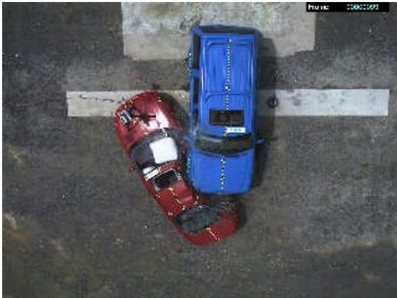
Figure 9: Overhead view of test 200 ms after impact (Test 10010) B-pillar impact
