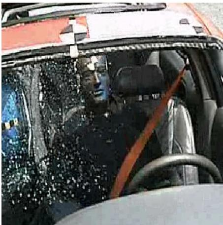
**Figure 17: Two frames from test 10010 showing the occupant-seatbelt contact at vehicle impact (above) and after 170 ms. (below)**
