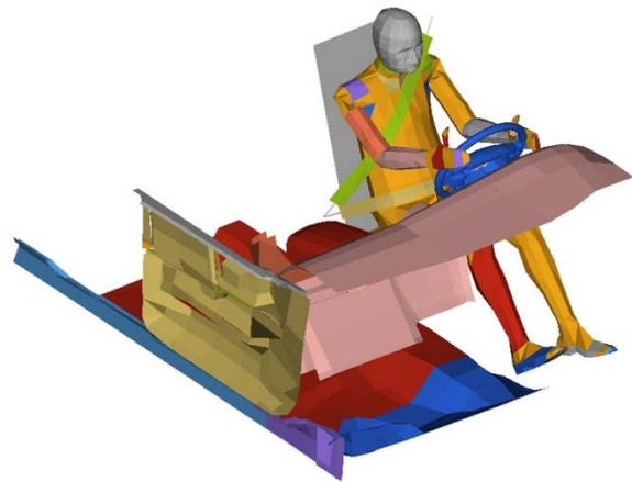
**Figure 7: The configuration of the MADYMO model for simulation of the two tests in the study**
