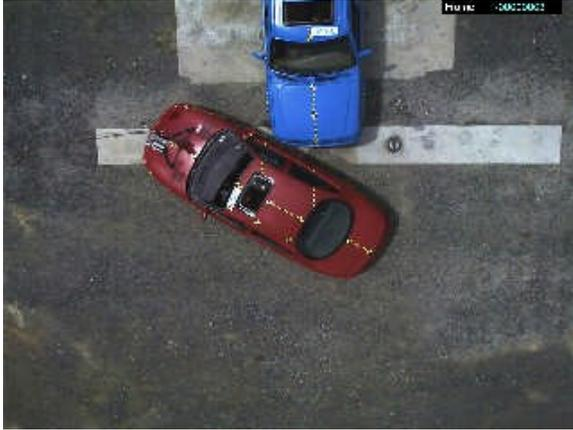
Figure 8: Overhead view of test at impact (Test 10010) B-pillar impact
