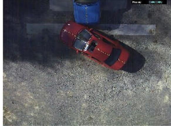
Figure 11: Overhead view of test at impact (Test 10016) A-pillar impact
