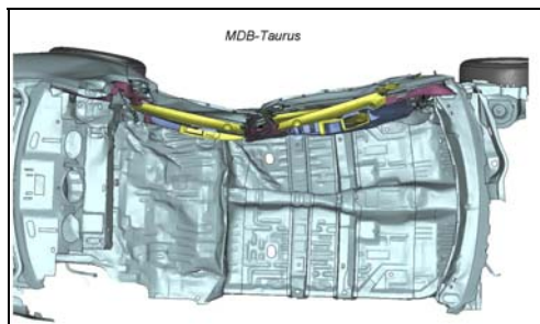
Figure 36. MDB-Taurus post-impact deformations.
