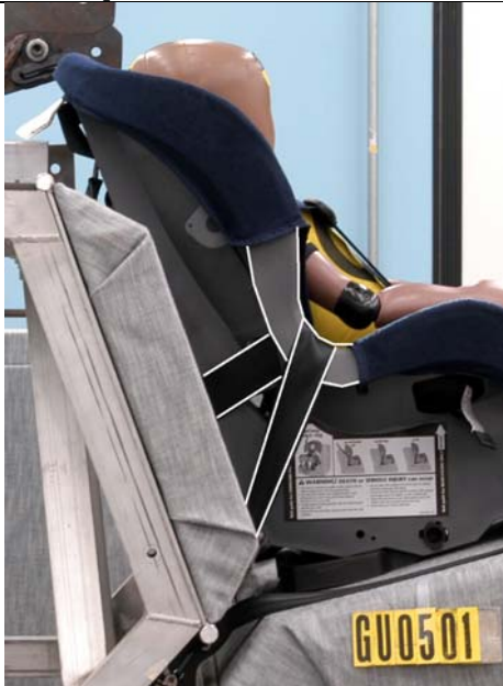
Figure 2. Annotated photo showing reverse belt routing used in test GU0501.
