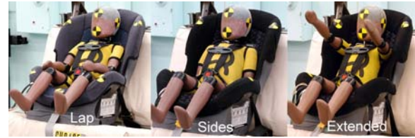
Figure 1. Initial ATD positions for tests varying arm posture: baseline with hands on lap (left), arms at sides (middle), and arms extended (right).
