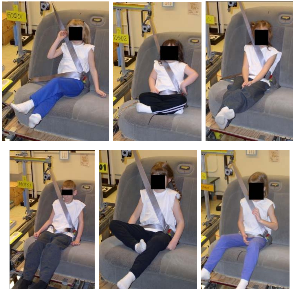
Figure 12. Photographs of sitter-selected-posture trials showing poor lap belt fit.
