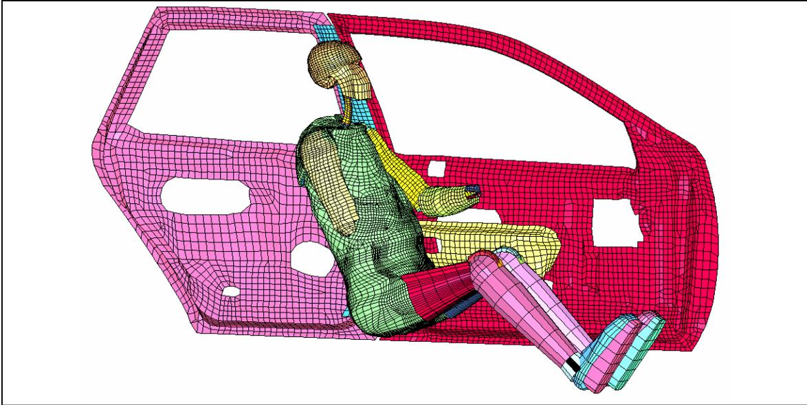
Figure 4: The door substructure and the whole-body human FE model in seating posture for Phase-2 simulation.
