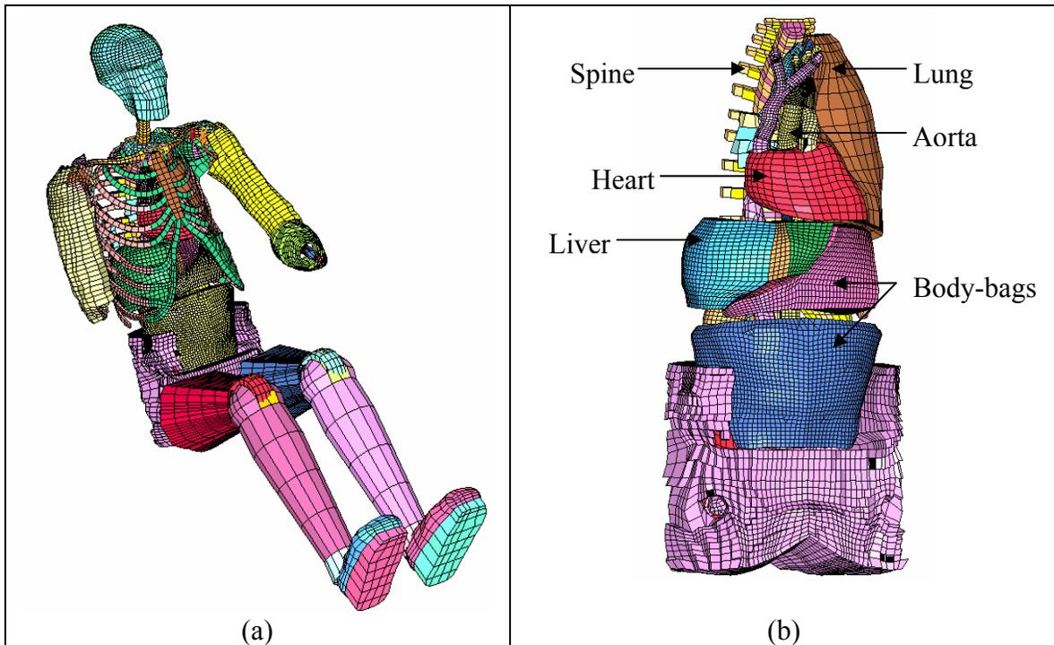
Figure 3: The whole-body human FE model (Shah et al. 2004).
