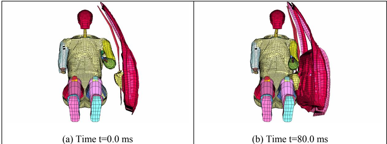
Figure 7: Interaction of the whole-body human FE model and the door structure for the Phase-2 simulation prior to impact and at the state of maximum door intrusion.
