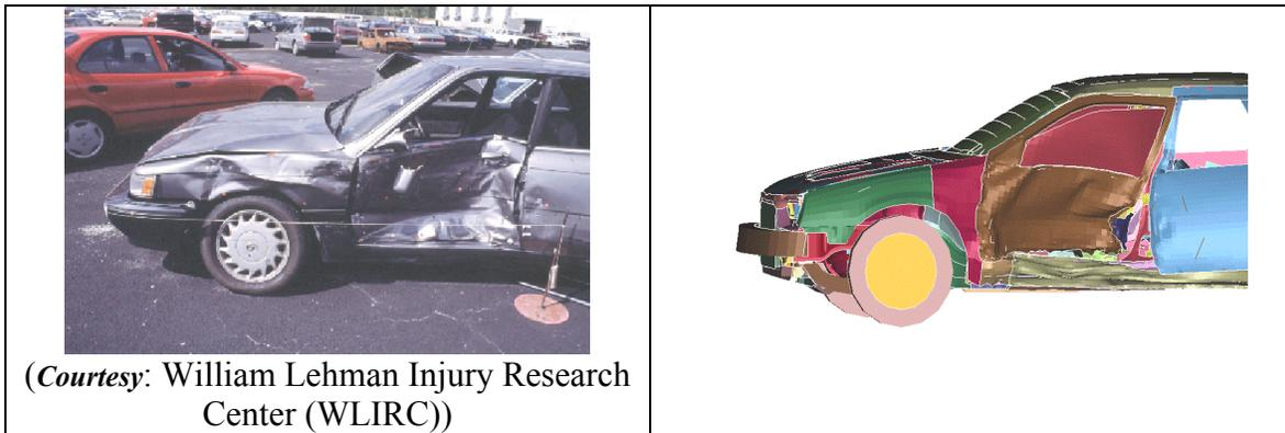
Figure 6: Deformation comparison between the real case vehicle and the FE vehicle model for Phase-1 simulation.
