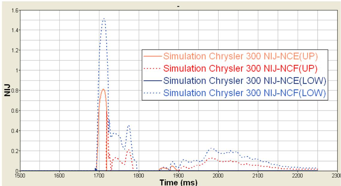
Figure 6 - Hybrid III Simulation NIJ
