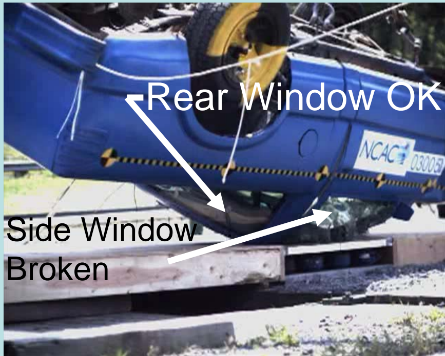
1 st Drop Maximum Roof Crush
