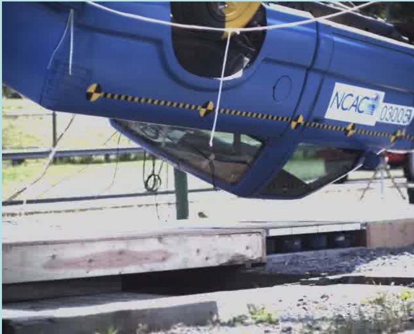
1 st Roof Impact
