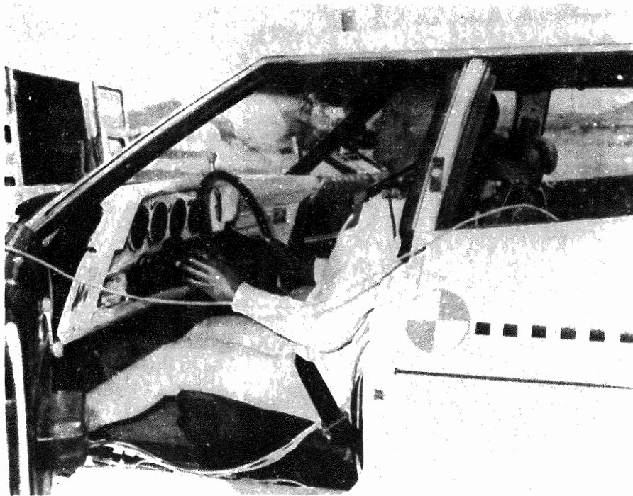
Figure 3-46. Pre-test Standard 3-Point Belt With Web Lockers and Force Limiters, Left Front - Test 14.
