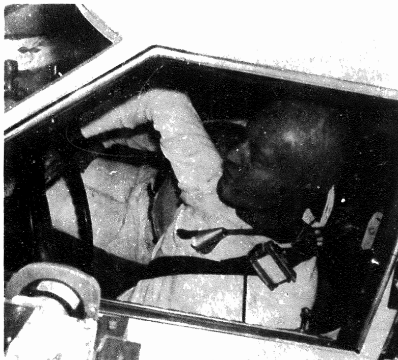
Figure 3-47. Post-test Standard 3-Point Belt With Web Lockers and Force Limiters, Left Front - Test 14.
