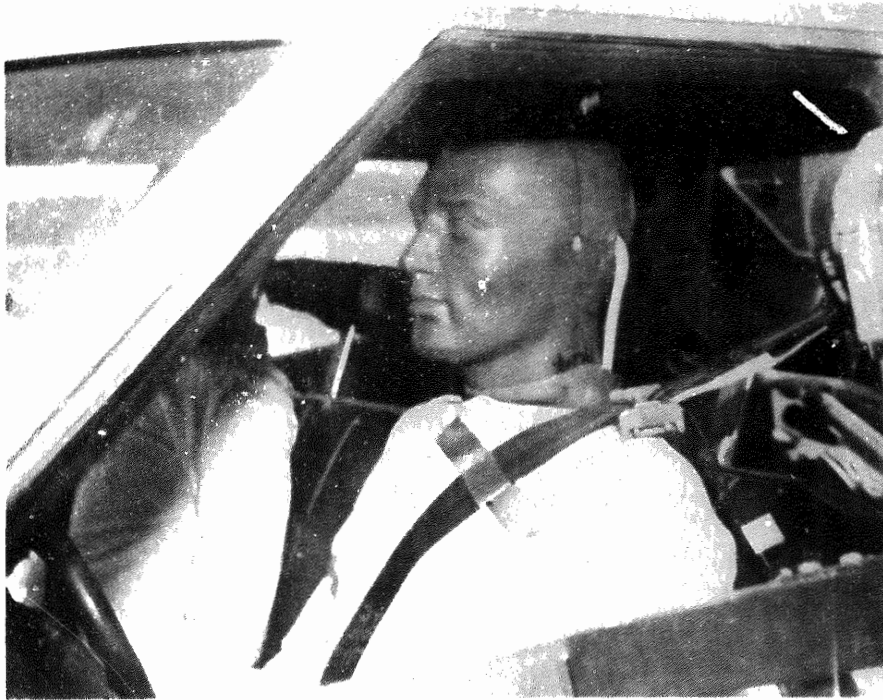
Figure 3-53. Pre-test Standard 3-Point Belt With Web Lockers and Tear Webbing, Left Front - Test 15.
