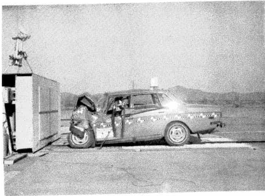
Figure 7-20. Vehicle Damage, Test 6-B
