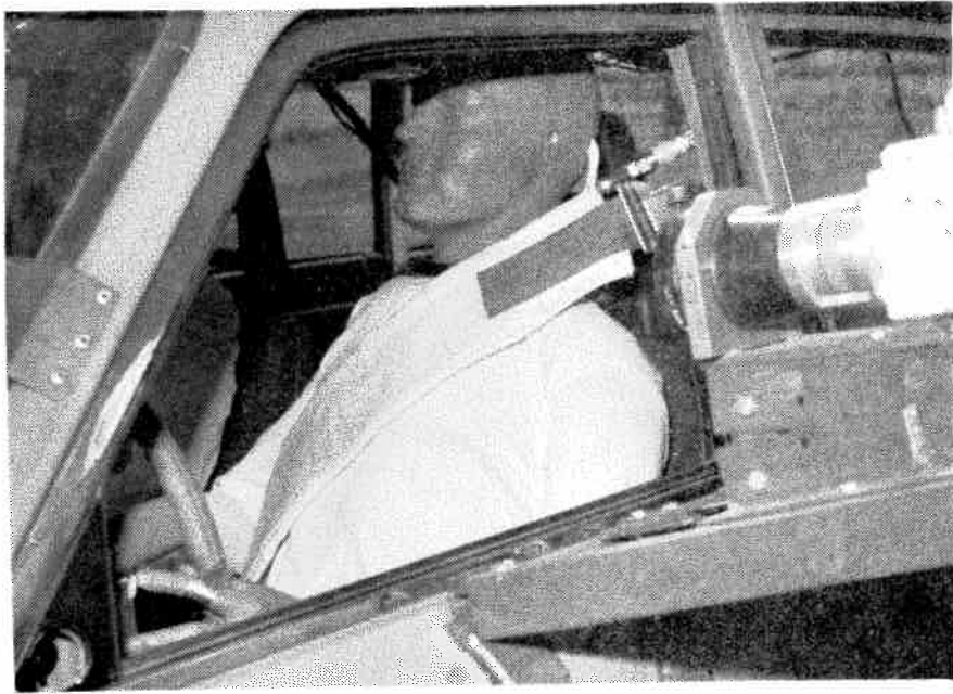
Figure 7-66. Airbelt System Prior to Test No. 17
