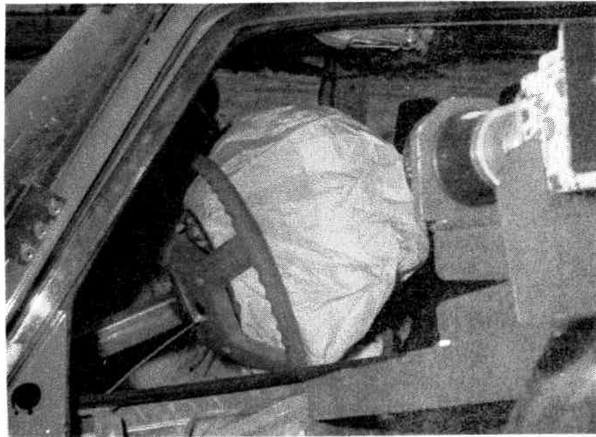
Figure 7-44. Driver System, Test No. 10
