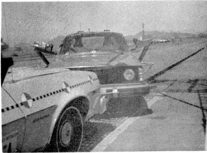
Figure 7-59. Test No. 14, 25 Degree Right Oblique
