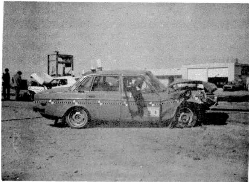
Figure 7-42. Volvo Damage, Test No. 10
