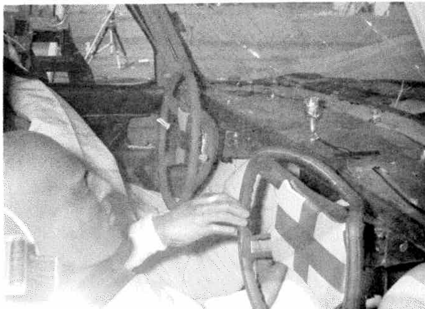
Figure 7-70. Wheel Rim After Impact with FLB Restrained Dummy's Head
