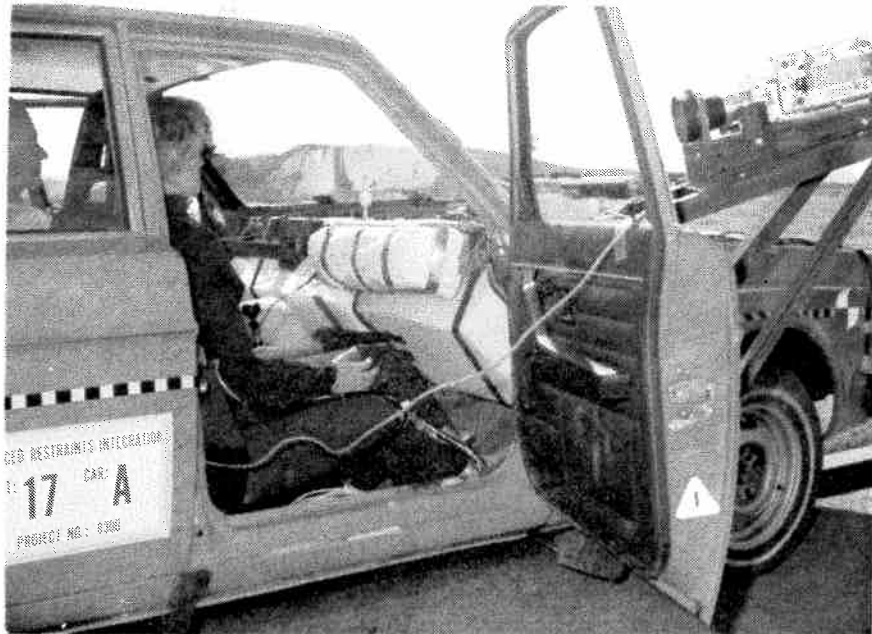
Figure 7-65. Passenger Airbag System Prior to Test No. 17
