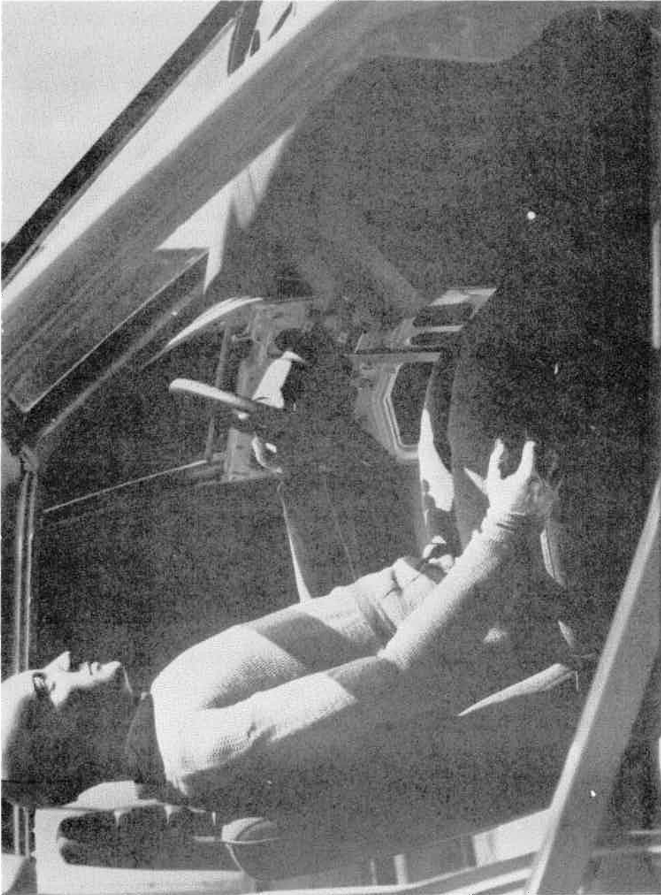
Figure 8-9. Driver Restraint System Installed in Buck
