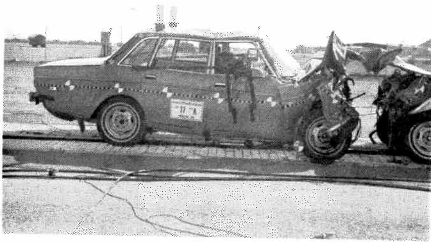
Figure 7-68. Volvo Damage, Test No. 17
