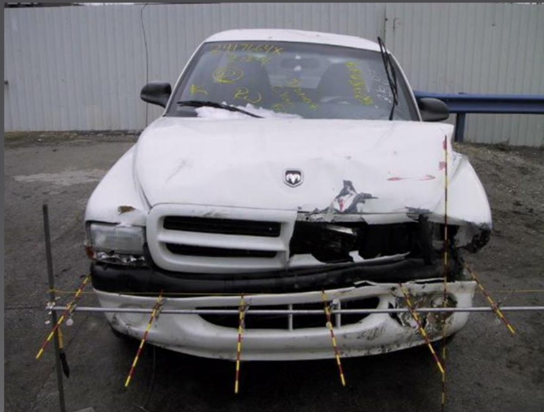
Low Severity Offset Crash – AIS 5 Chest Injury Driver with severe coronary atherosclerosis NASS Case 2004 73 42 1
