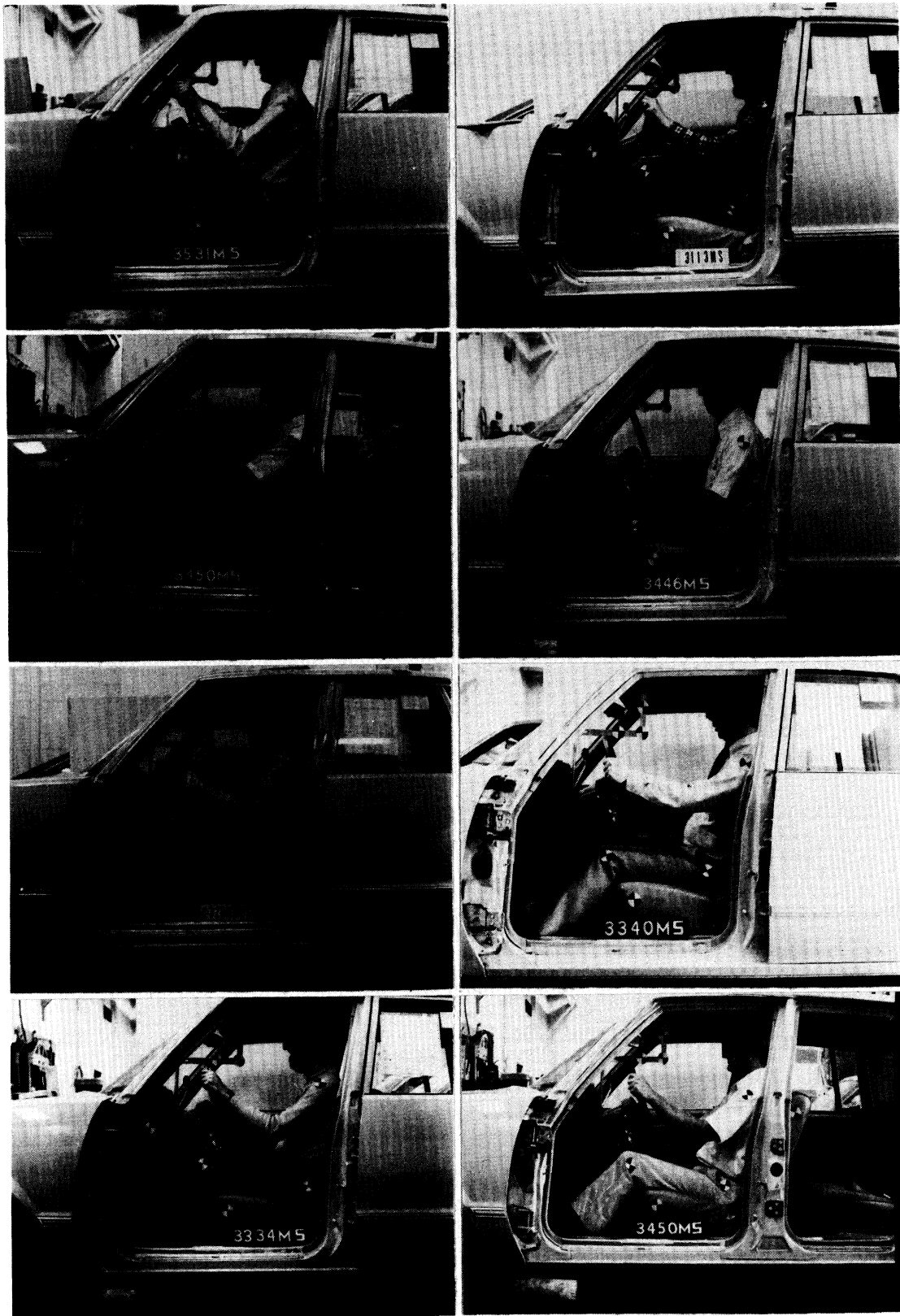
FIGURE A-3. Examples of the "standardized normal driving posture" for eight mid-sized males in the Chevrolet Malibu.
