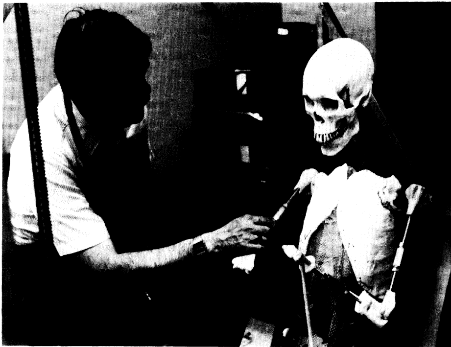
FIGURE 4-2. Adjustable skeletal armature used for mid-sized male clay model.
