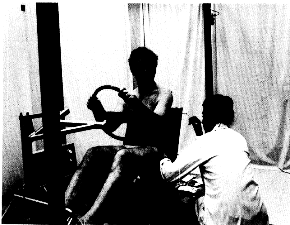
FIGURE 3-29. Contrast targets being placed at surface landmarks on seated subject.
