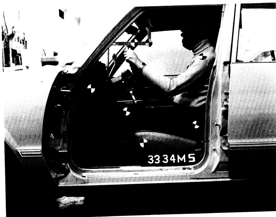
FIGURE 3-3. Mid-sized male subject sitting in Malibu showing little or no difference between "normal" (above) and "standardized" (below) seated postures.
