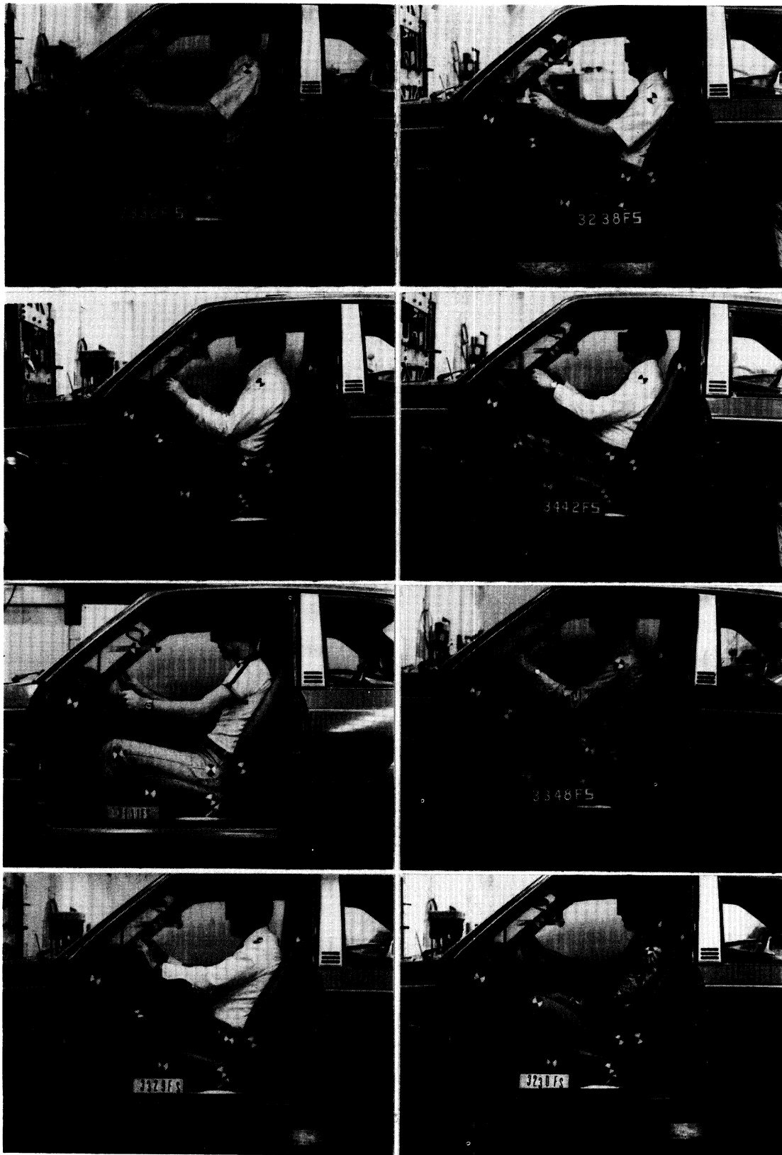
FIGURE A-4. Examples of the "standardized normal driving posture" for eight mid-sized males in the Ford Escort.
