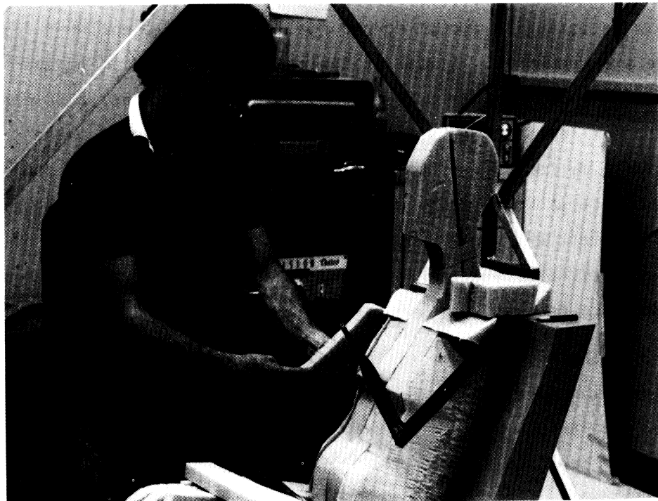
FIGURE 4-4. Attaching styrofoam to welded steel armature.
