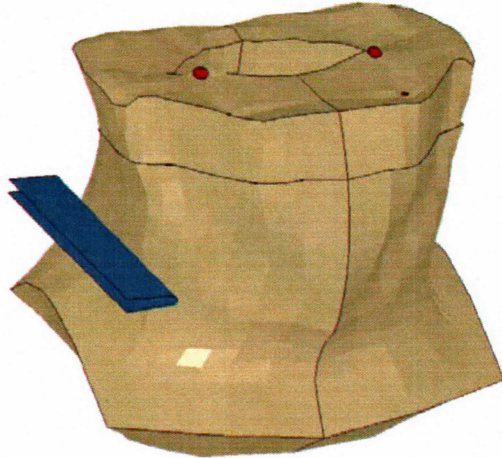
Figure 2.1-1: Initial neck regional model with neck fascia, carotid arteries and a seatbelt indenter.
