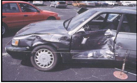
Figure 2. Case vehicle for a 22.5 km/h (14 mph) crash resulting in aortic tear.
