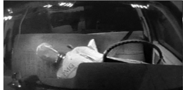
Figure 3. Dummy Position at Maximum Lap Belt Loading
